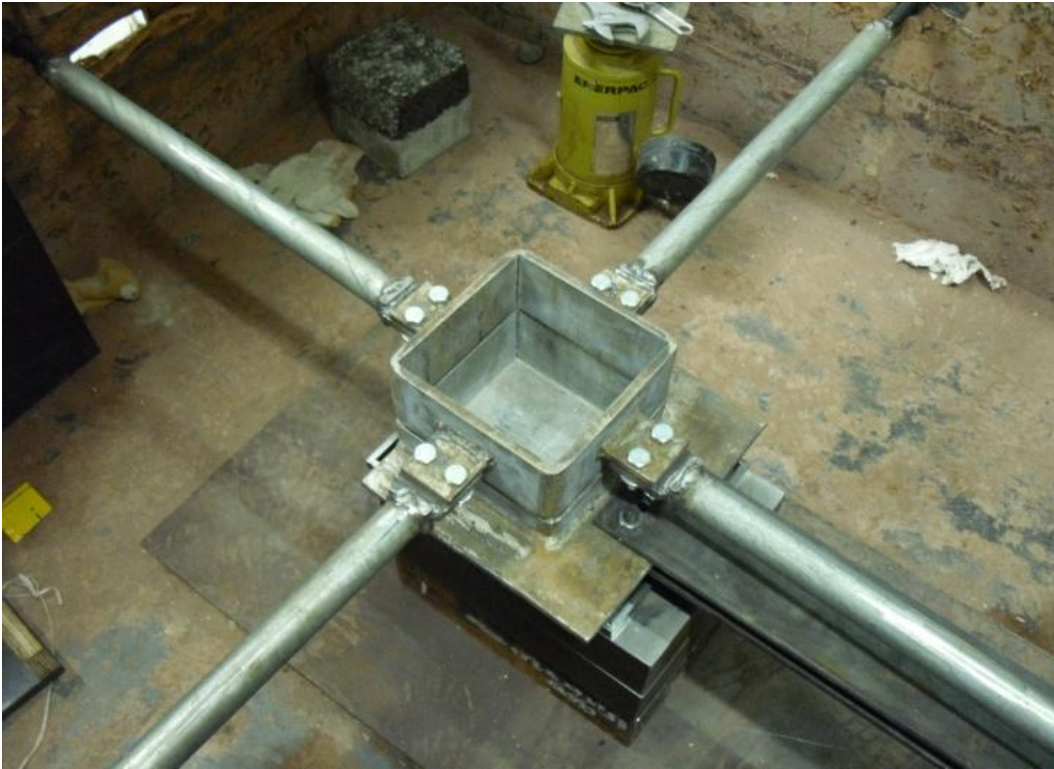
(b) Upper box fixed by steel bar
