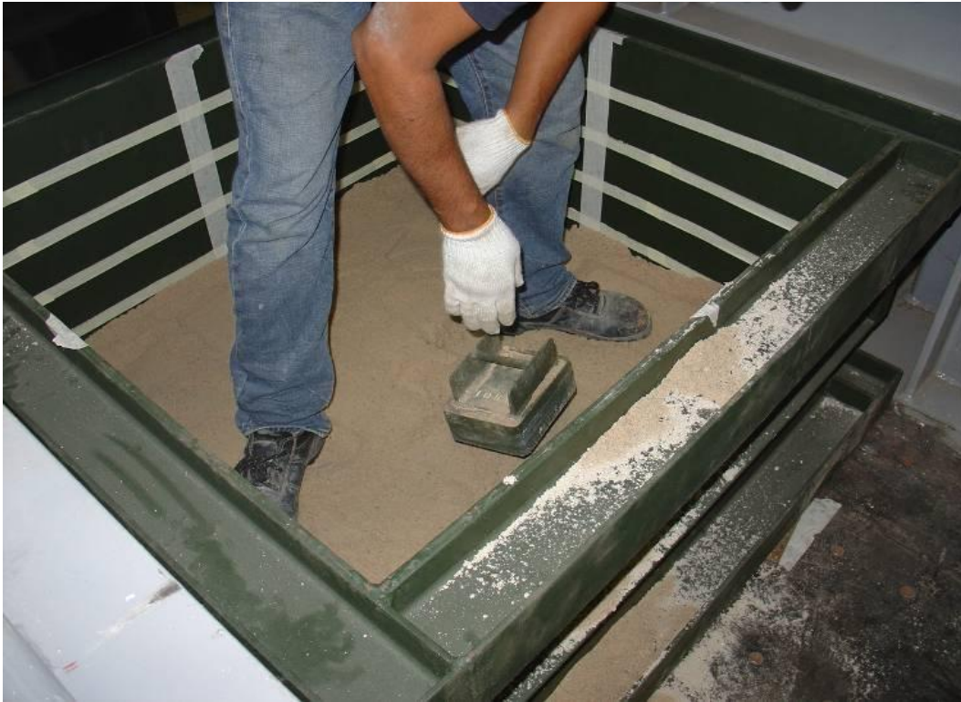
Figure 3.5 Compacting of sand in steel strong box
