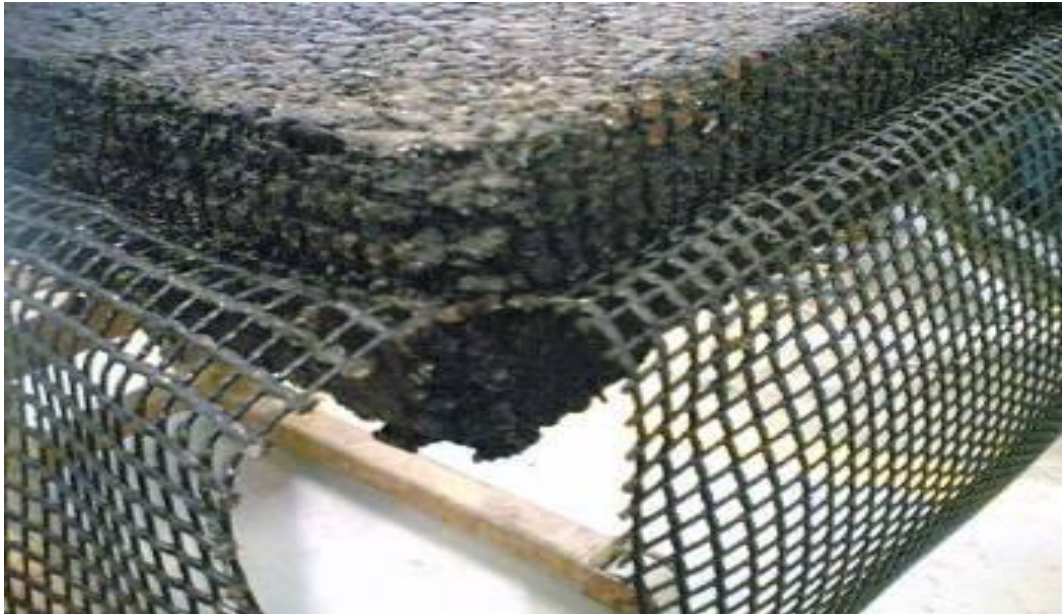
Figure 2.27 Geogrid Installed in Asphalt Layer (after Yong 2005)
