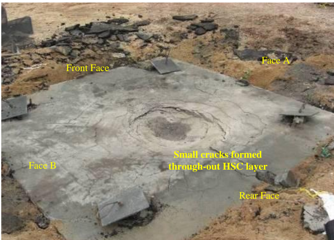
Figure 4.37 Crater details for Slab 2 after removal of asphalt layer
