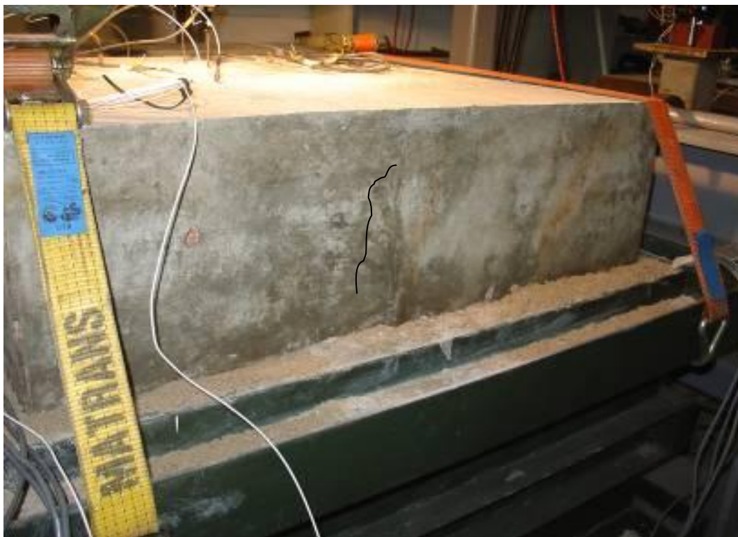
Figure 3.13 Crack Propagation in Sample A after 1 st Impact
