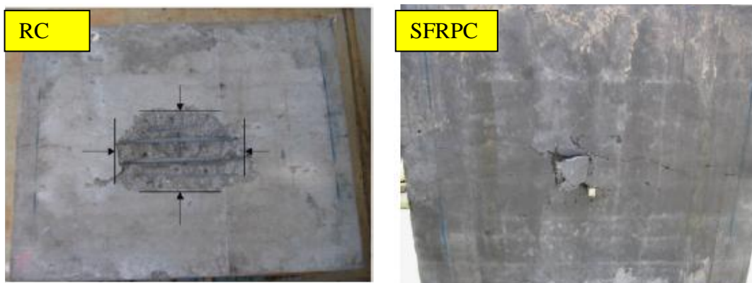
Figure 2.21 Experimental results of RC and SFRPC under bare charge (bottom surface) (after kuznetsov et al. 2006)
