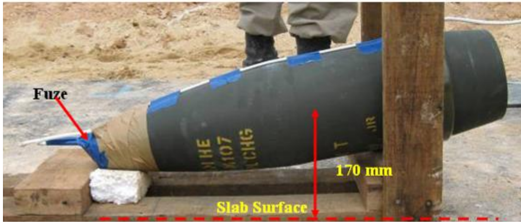
Figure 4.1 M107 Placement on Slab
