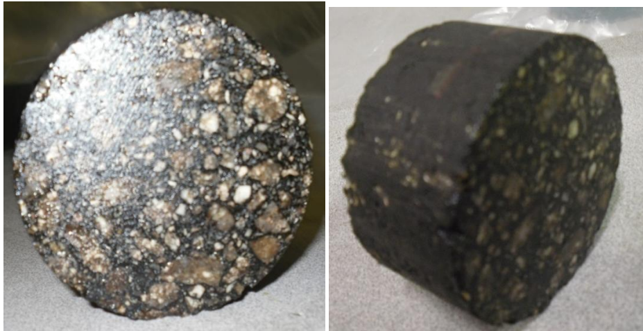
Figure A.3 Asphalt concrete specimen with lubricating surface for SHPB test
