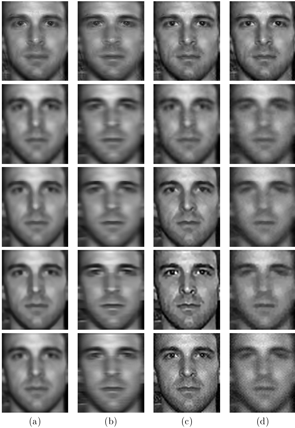
Figure 7.17: Superresolution (1 st row), bilinear (2 nd row), neighborhood embedding method [21] (3 rd row), fast image upsampling method [77] (4 th row), and sparse representation method [99] (5 th row) on images with different blurs and noise: (a) Blurry image from a 5 \times 5 averaging mask, (b) Blurry image from a motion blur filter, (c) 20db noisy image (d) Image with combined effects of (a), (b) and (c).
