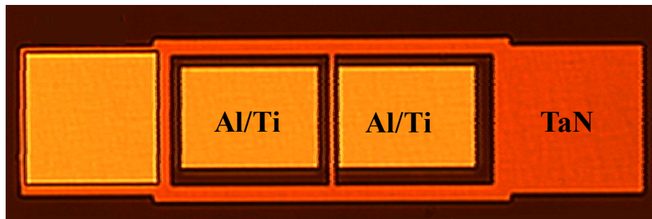
(e) Optical image of the fabricated TaN/HfAlO/GaN capacitor.
