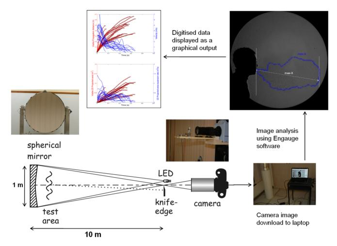
Figure 1. Experimental set-up for the shadowgraph imaging of the human respiratory airflows described in this study (reproduced from Tang et al. 2012). doi:10.1371/journal.pone.0059970.g001
