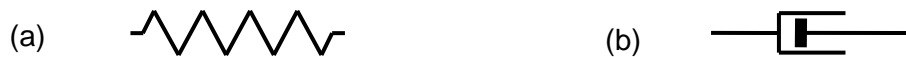
Figure A.1 Basic elements of viscoelastic models. (a) Linear spring and (b) linear dashpot.
