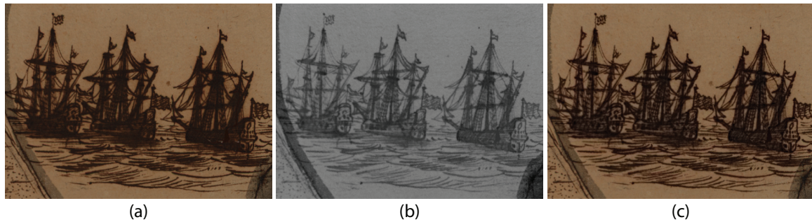
Figure 1.2: An example of the visual enhancement of old documents: (a) original RGB image; (b) 850nm NIR band image; (c) enhanced result.
