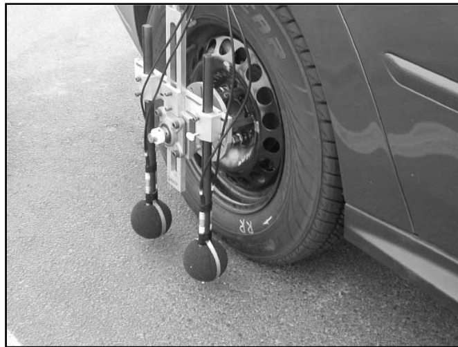
Figure 2.18 Onboard sound intensity measurement system (ASTM, 2009)
