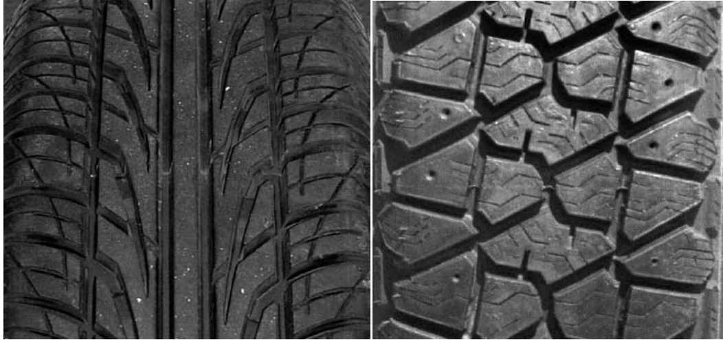
Figure 2.17 CPX reference test tires (Avon/Copper and Dunlop) (Roo et al., 2009)
