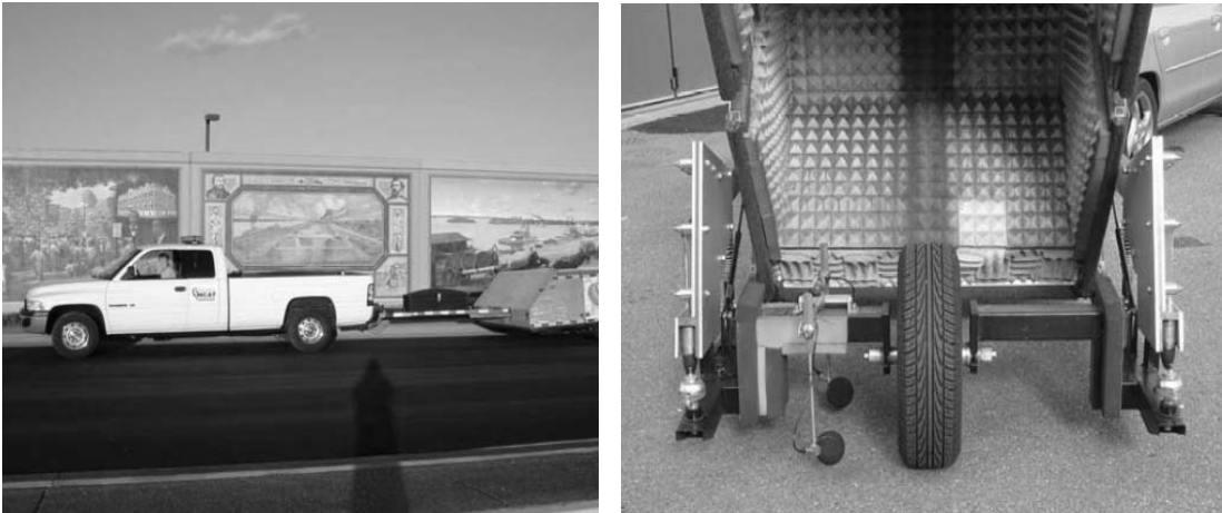
Figure 2.15 CPX trailer measurement equipment (Roo et al., 2009)
