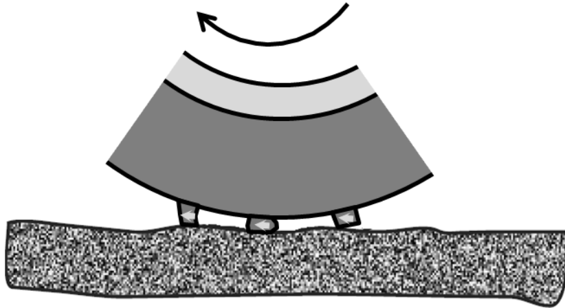
Figure 2.3 Stick-slip noise generation mechanism
