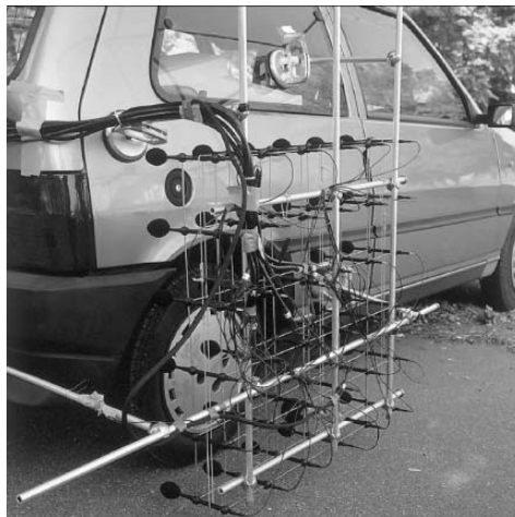
Figure 2.20 Microphone array positioning for tire noise measurement on a moving vehicle (Rasmussen and Gade, 1996)
