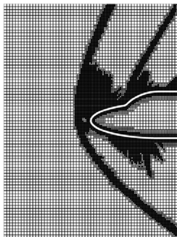
(b) Solution adaptive mesh (2x), pressure contours and streamlines computed by LDFD-IBM.
