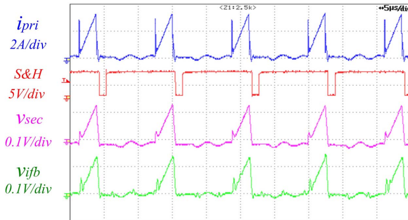
Fig 4.17: Current Sensing Operating Waveforms (experiment)
