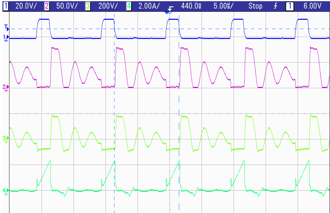
(a) DCM operation V_{pv} = 25V, V_g = 200V, D = 19.8\% (Ch1: v_{gs} ; Ch2: v_{ds} ; Ch3: v_{sec1} ; Ch4: i_{pri} )
