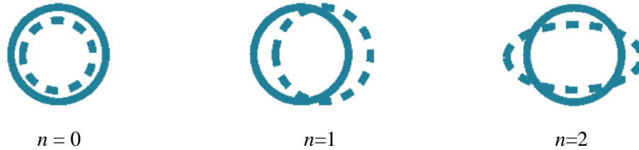
Figure 5.5 Branching of an electrospun jet can be considered as a complex mixture of azimuthal mode n , where n is 0, 1 and 2.
