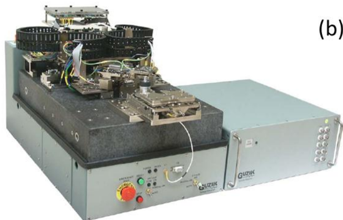
Figure 4 - 3 (a): M7 error analyzer add-on board for the Guzik spin-stand Figure 4 - 3 (b): Guzik spin-stand DTR3004 setup
