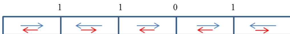
Figure 1 - 5: Longitudinal recording and its respective media bit orientation and detected transitions, where demagnetization fields are denoted by the smaller red arrows
