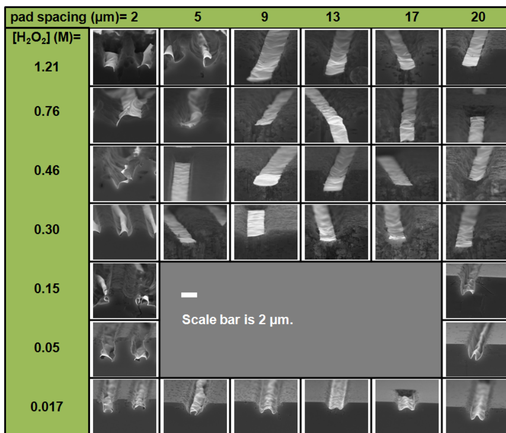
Figure C1: Cross-sectional SEM images of the etched samples used to construct the stability diagram in Figure 4.17 . [HF] was fixed at 1.73 M.
