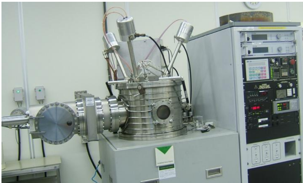
Figure 2.5: Overview of a Denton sputtering system.
