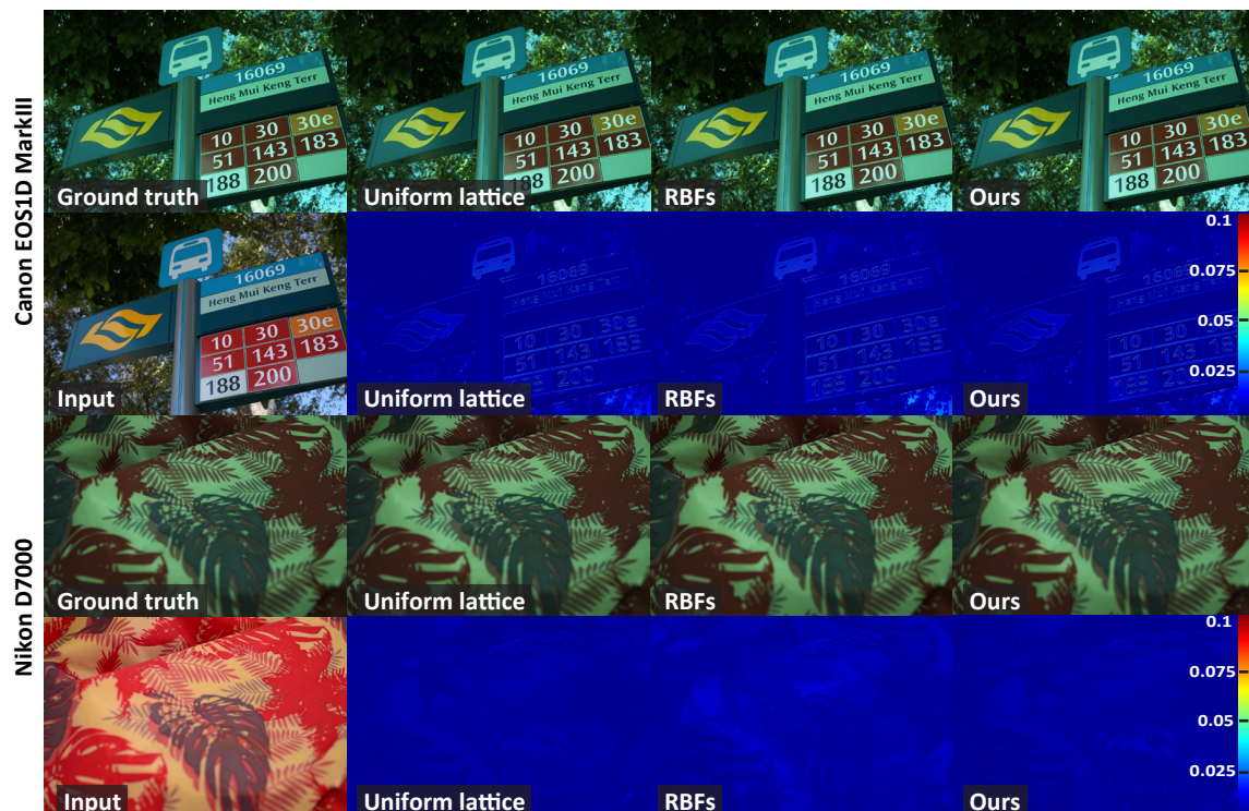
Figure 5.6: Comparing the results of transforming images in sRGB back to their RAW images. The input Canon image is of standard picture style and sunny white balance, while the Nikon input image is of landscape picture style and shade white balance. The error maps between our method, RBFs, and an LUT based on uniform lattice regression [19] are shown, from which we can see that since the input space is not very skewed, the uniform lattice method produces comparable results as our method and RBFs. Noted that the intensities of RAW images are stretched for visualization purpose.
