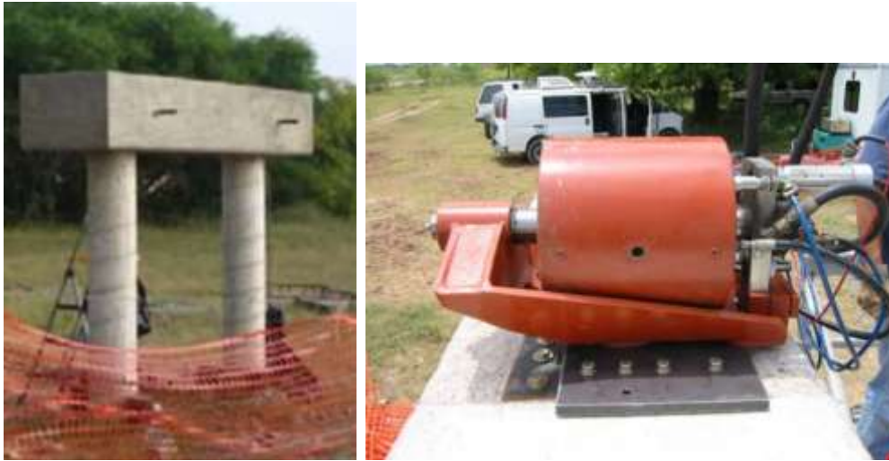
Figure 2-3 Harmonic excitation using shaker from Thumper (Agarwal et al. , 2010)
