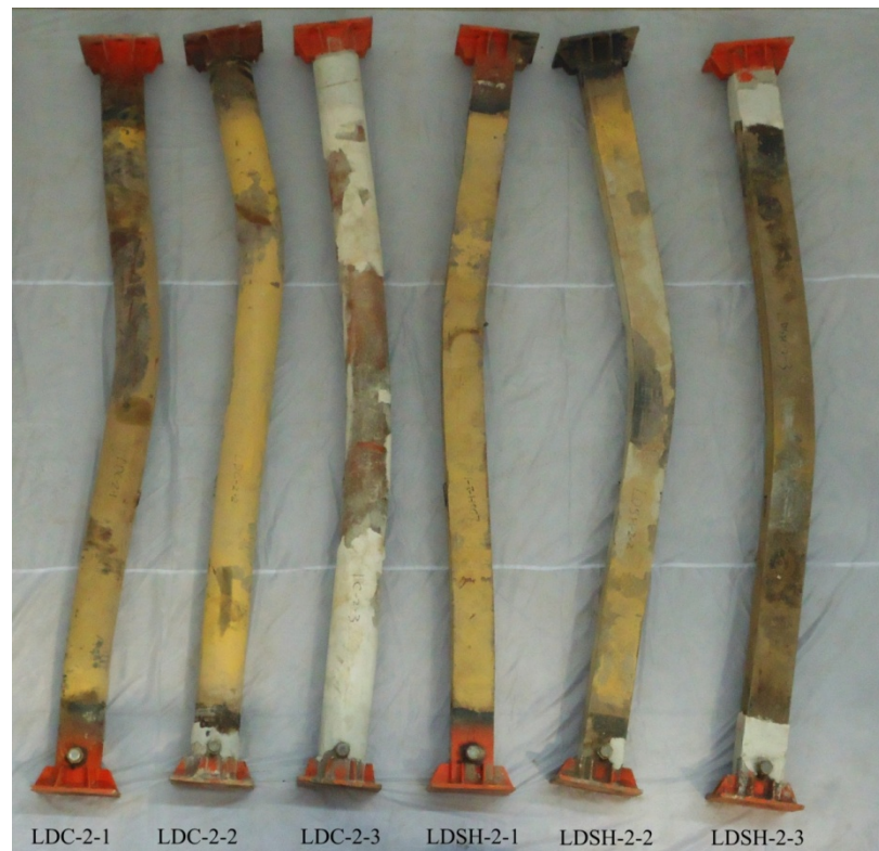
Figure 6.26: Comparisons between failure modes of double-skin columns
