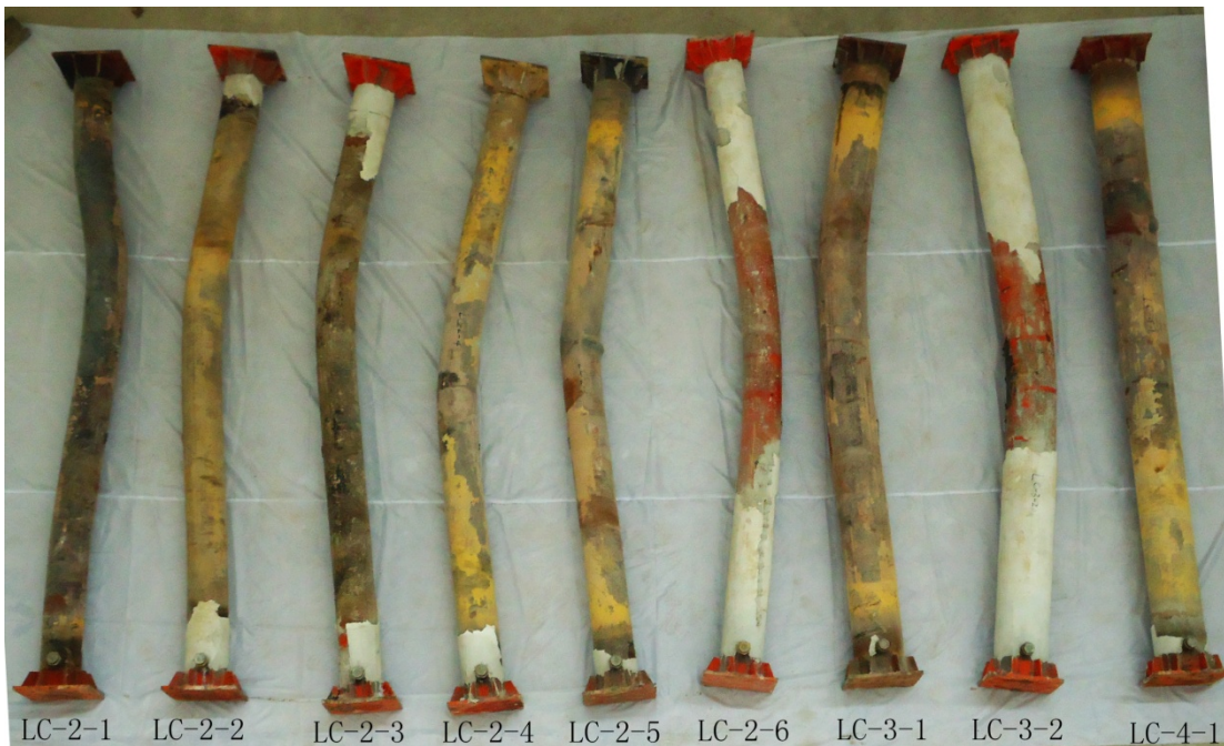
Figure 6.24: Comparisons between failure modes of circular single-tube columns
