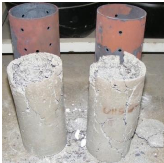
Figure 4.3: Spalled UHSC specimens with steel fiber after taken out from oven
