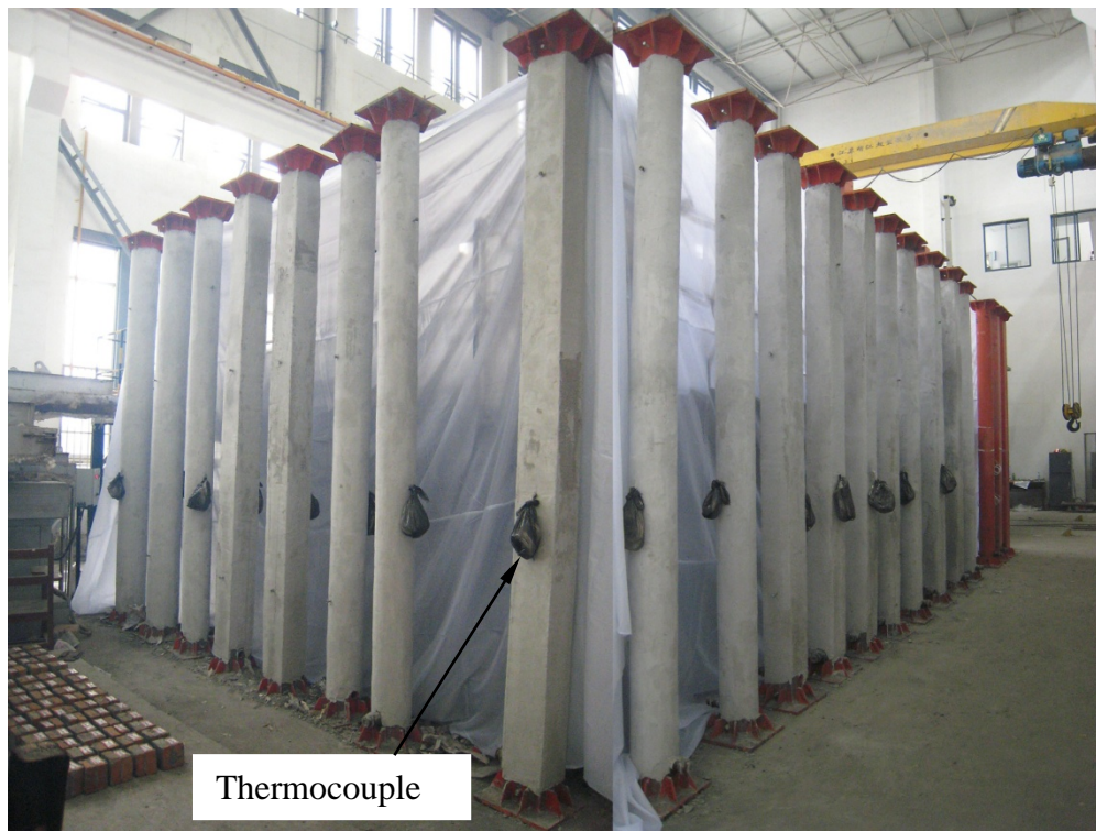
Figure 6.10: CFST columns applied with fire protection material
