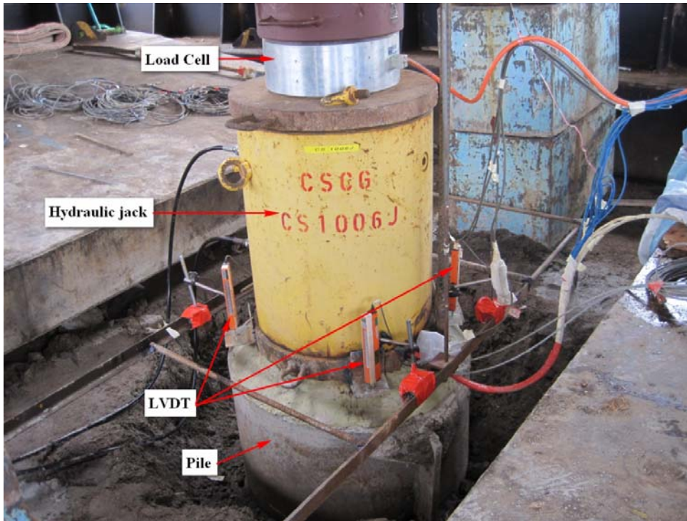
Figure 5-26 Photo of the experimental set-up for static pile load test.
