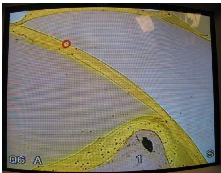
Fig. 4.4 An optical microscope image ( \times 10 magnification) displayed on a monitor, of an aggregate of octahedral particles, with a mean edge length of l = 78 nm, illuminated by white light. The microscope is optically interfaced with the BLS system. The gold particles appear as yellow regions, while the other regions represent the exposed silicon wafer which served as the sample holder.
