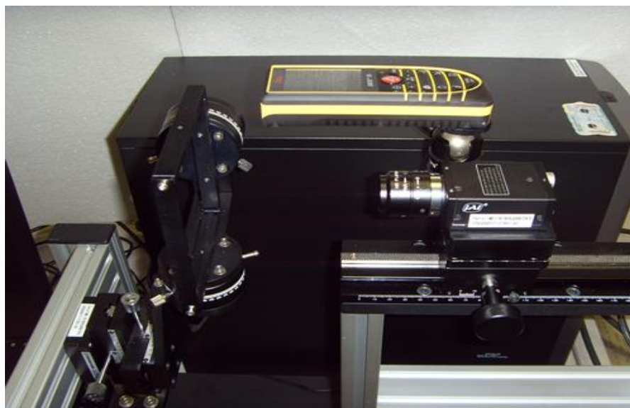
Fig. 5.1: Experimental setup of the single-lens prism based stereovision system
