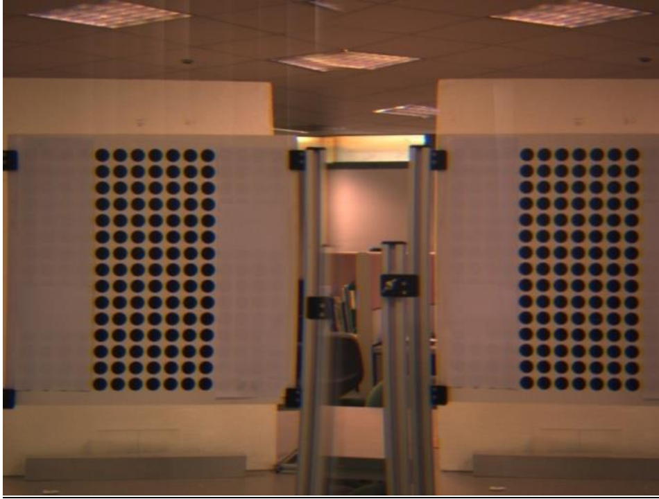
Fig. B.3: Experimental stereo image pair taken at distance 1800mm
