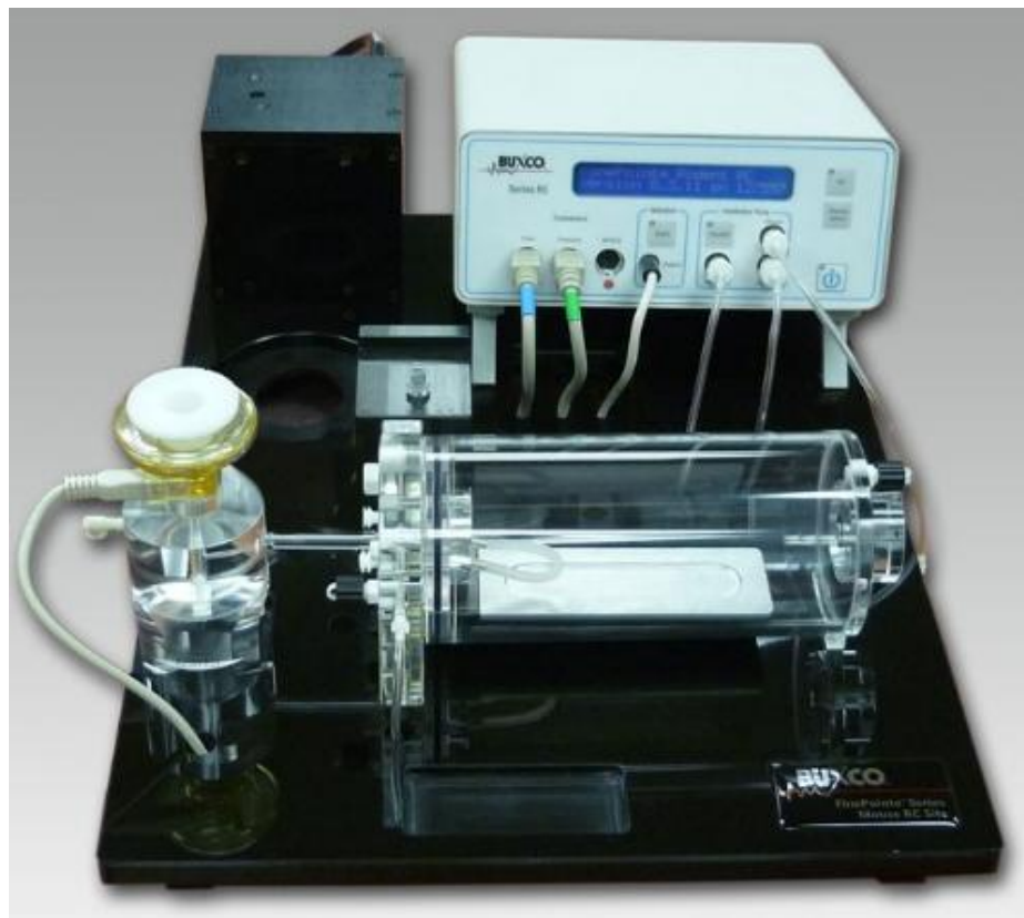
Figure 3.5. The FinePointe™ system (Buxco Research Systems, Wilmington, NC, United States). The system measures the resistance and compliance of mouse in response to aerosolized methacholine. The system comes with in-line aerosol, ventilator, and heated bed.
