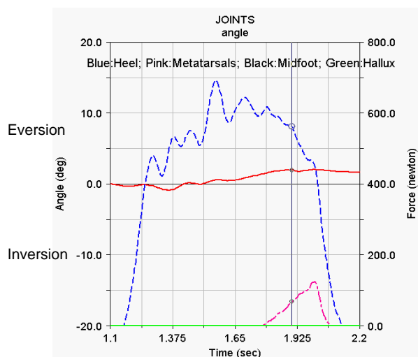
Figure 7.40: Shank-Heel coronal plane angle feature (solid, red line) VS contact forces (Walking with Weights)
