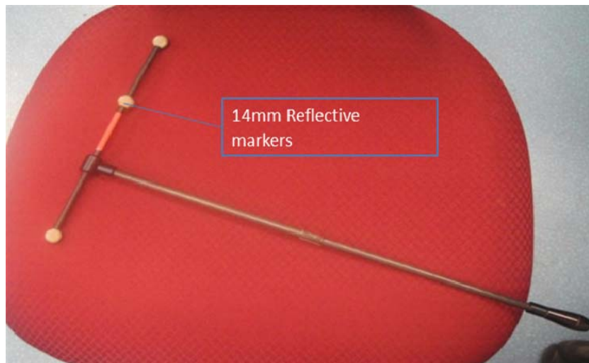
Figure 5.5: Standard wand with three reflective markers for dynamic calibration
