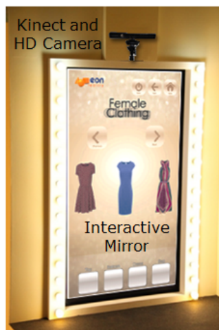
Figure 4.1. The front view of the Interactive Mirror with Kinect and HD camera placed on top.
