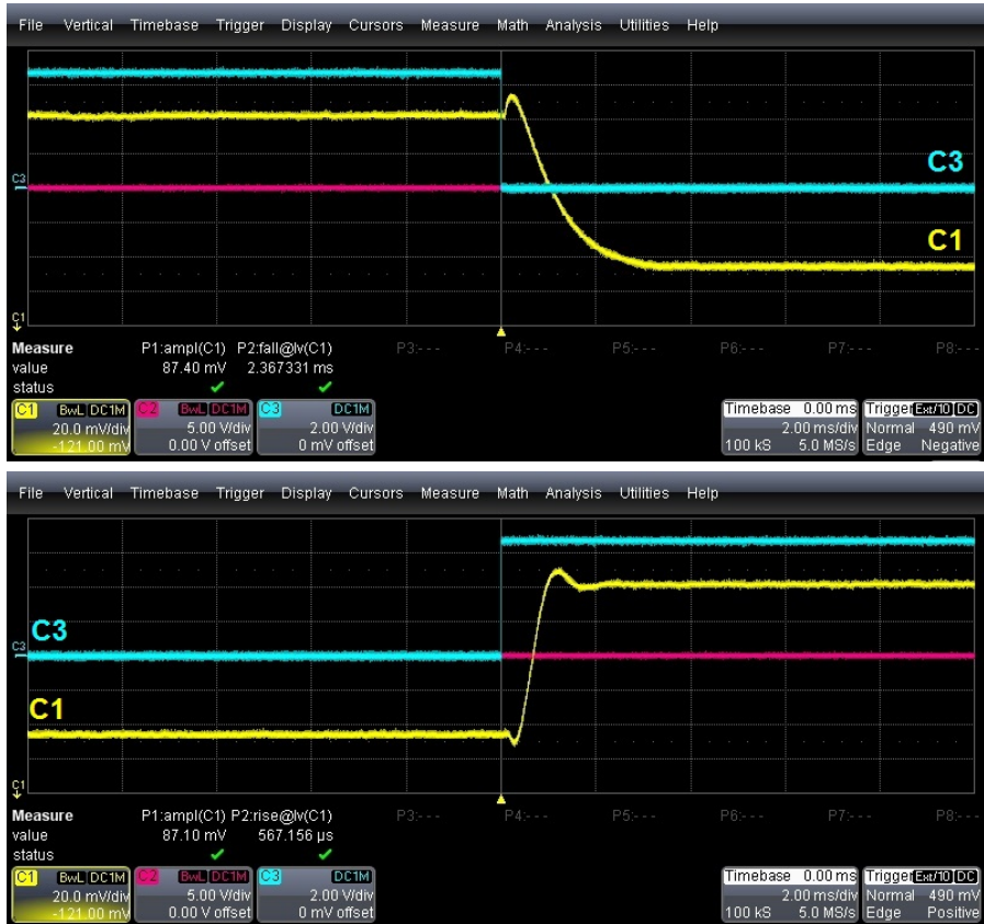
Figure 42: Oscilloscope trace of magnetic field in the x-direction when switching off the quadrupole field. The cyan trace (C 3 ) is the trigger for the switch while the yellow trace (C 1 ) is the field probed with a fluxgate magnetometer (Stefan Mayer FLC 100). The red trace is unused. A full switch-on time of ~ 2 ms and a switch-off time of ~ 4 ms were measured. The magnetometer, which has a maximal bandwidth of 1 kHz and range of ±1 Gauss, is placed along the quadrupole x-axis and at a distance away such that it does not reach saturation. During switching of the magnetic field coils, about ~ 10–20 ms is given to allow the magnetic fields in the coils to stabilise.
