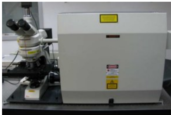
Fig 2.13 Renishaw 2000 Raman/PL microscope set up
