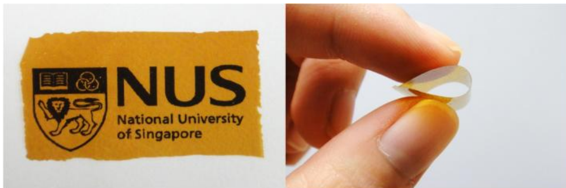
Figure 4.4 The appearance of 50/50 (w/w) ZIF-7/PBI nano-composite membrane Left: Tiled on an NUS logo; Right: Bended with fingers.
