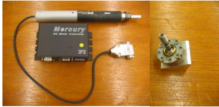
Figure 9.6 The M-235.5 DG Actuator and Hephaist Seiko Spherical Joint
