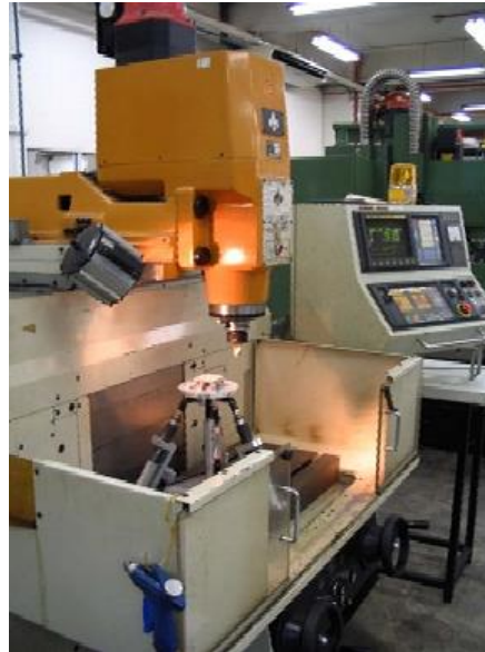
Figure 9.18 Integration of the hybrid 3-DOF PKM into 3-axis machining center
