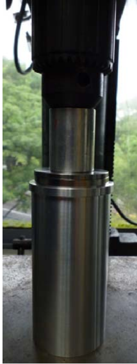
Figure 48: Bench Drill Used to Press the Magnet-Spacer into the Outer Casing
