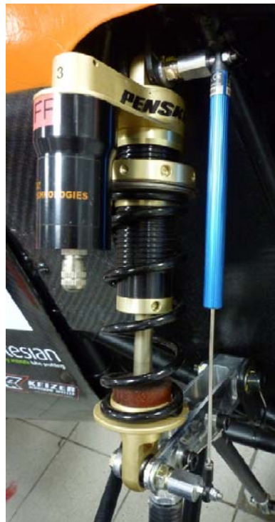
Figure 1: Linear Potentiometer on NUS Formula SAE 2012 Race Car Damper
