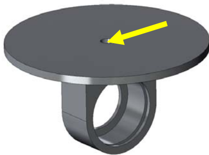
Figure 60: Lower Bearing Mount (Left) with Arrow Showing Tapped Hole Location, Bolt Inserted into Lower Bearing Mount Badly Slanted
