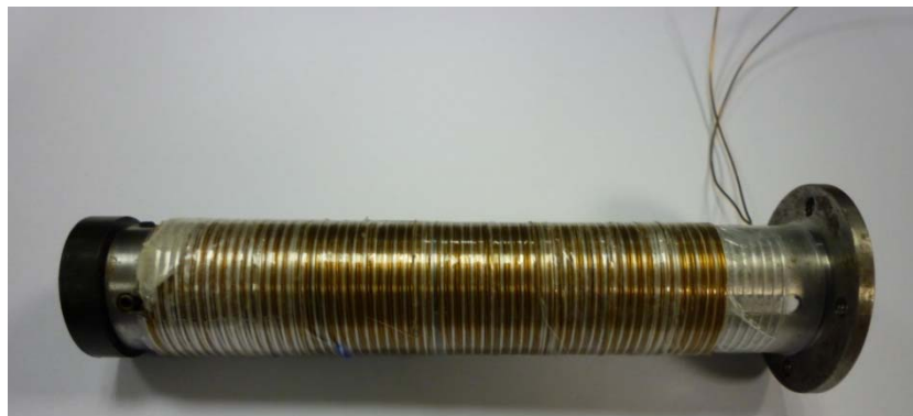
Figure 50: AWG 18 Wire Coil on Wire Coil Housing
