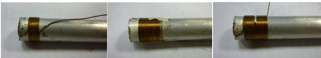
Figure 38: 10 Turns Clockwise (Left), 20 Turns Clockwise (Middle) and 10 Turns Clockwise and 10 Turns Anticlockwise Wire Coils (Right)
