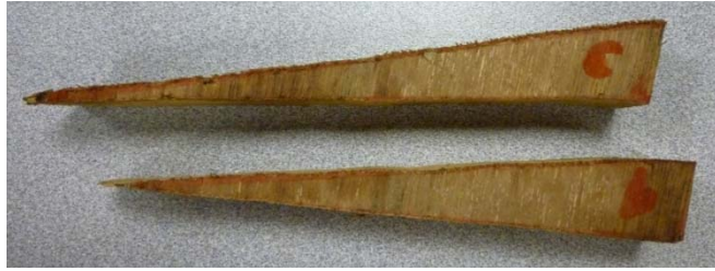
Figure 46: Wedge Made of Wood to Ease the Magnet to the Spacer
