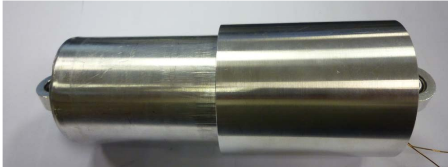
Figure 51: Electromagnetic Damper Fully Assembled
