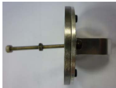
Figure 60: Lower Bearing Mount (Left) with Arrow Showing Tapped Hole Location, Bolt Inserted into Lower Bearing Mount Badly Slanted
