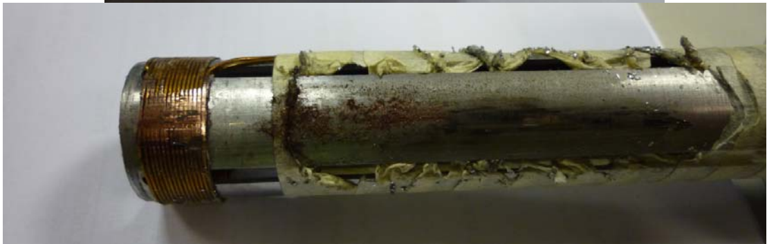
Figure 59: Enamel Wires Being Scrapped (Top), Zoom In of the Damage (Bottom)
