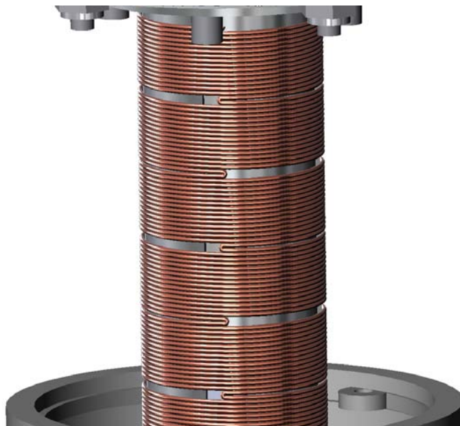
Figure 36: CAD of Wire Coils Changing Direction
