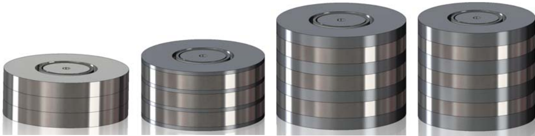
Figure 28: Various Ferrous Spacer Analysis, No Spacer, Quarter Spacer Height, \frac{3}{4} Spacer Height and Same Magnet Height, Left to Right
