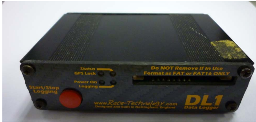
Figure 55: Race Technology DL1 Data Logger
