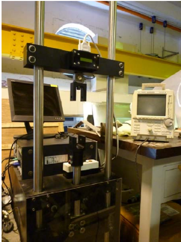
Figure 52: Damper Dynamometer (Left) and Cathode Ray Oscilloscope (Right)
