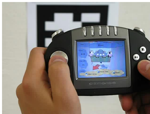
Figure 8. A computer vision-based handheld augmented reality game where a physical marker is required to be in view of the device's camera. (Source: Mulloni and Wagner, 2010.)
