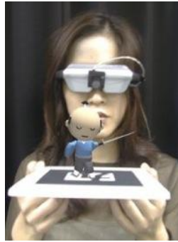
Figure 3. A 3D model on a fiducial augmented reality marker seen through a head-mounted display. (Source: Kato and Billinghurst, 1999)
