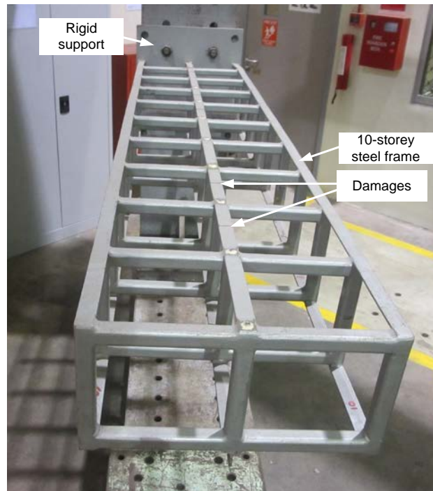
Figure 3.10 The 10-storey steel frame
