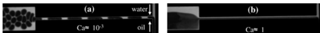
Figure 2.6. The effect of capillary number on the flow pattern of oil and water phase. The capillary number was tweaked by changing the interfacial tension by means of surfactant and keeping other parameters flow rate ratio, viscosity ratio constant. Droplet flow pattern on the left at Ca \sim 10^{-3} and stratified flow pattern at Ca \sim 1 on the right can be observed (Shui et al., 2008).
