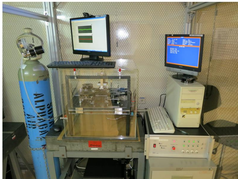
Figure 9-1 Wear tests setup enclosed in the environmental chamber connected to pure dry air cylinder
