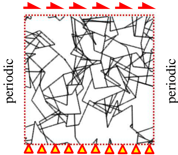
Figure 4.1: Initial configuration of a typical network. Dangling ends are removed and the boundary of the computational window (red dashed lines) along with the b.c.'s are shown.
