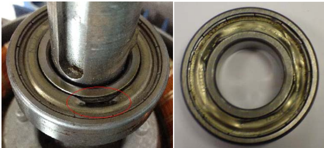
Fig. 2.2 Fault located on the bearing
