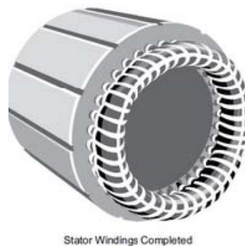
Fig. 2.1.1-b) The stator of an induction motor [6]
