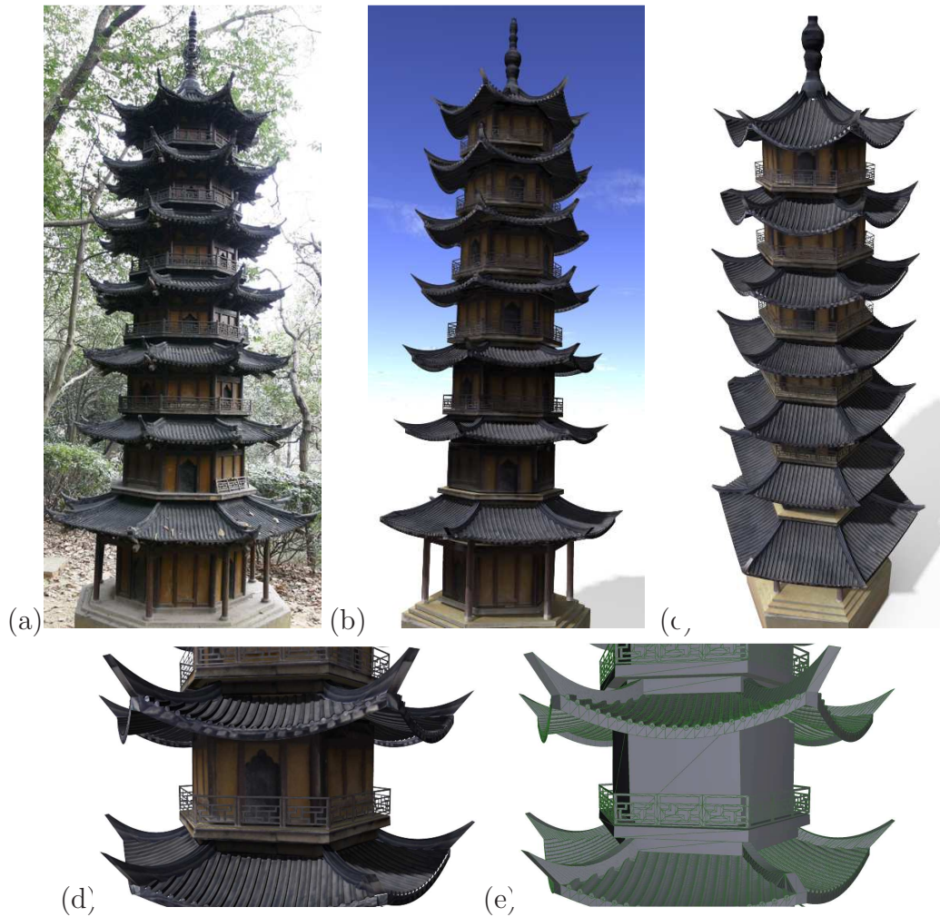
Figure 5.12: A pagoda with highly curved roof. Each roof is different from the others. (a) is the single input image. (b) is the recovered model rendered from the same view as the input image. (c) is the rendering from a novel viewpoint. (d) shows a close-up view of the building. (e) is the shaded wireframe to highlight the geometry. (Please zoom in the electronic version.)
