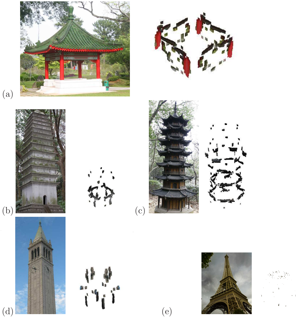
Figure C.1: Reconstructed 3D points from symmetry-based stereo. (a) The Pavilion example. (b) and (c) are two pagoda examples. (d) and (e) are results obtained for Berkeley Campanile and Eiffel Tower, reconstructed 3D points are relatively few for these two examples. This could be explained by matching failure on the textureless façade of Berkeley Campanile and bad correspondences between the rectified views of the curved façade of Eiffel Tower (which violates the homography transformation assumption between frustum faces).
