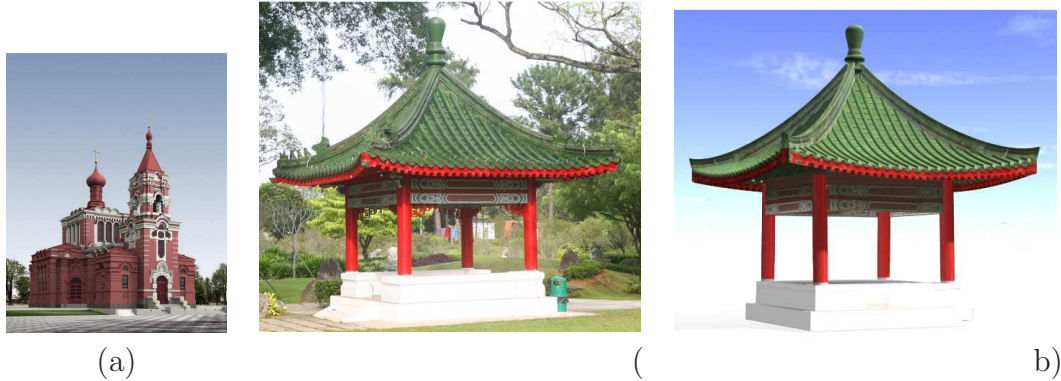
Figure 5.1: Architecture models created using modeling software and image-based modeling algorithm. (a) Church model created from 3dMax. (b) A pavilion modeled using our proposed modeling method. On the left is the single input image. On the right is the recovered model rendered from the same viewpoint as the input image.
