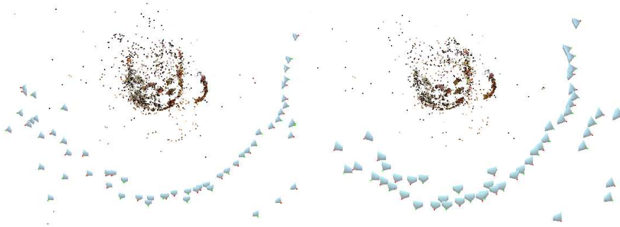
Figure 3.1: The middle of first row shows the true configuration in which multiple images are captured around a cup. We highlight a pair of correct and incorrect image matches in the green and red rectangles respectively. The second row are the reconstructions obtained using (83) and (99) respectively. All cameras are incorrectly reconstructed on one side of the cup.
