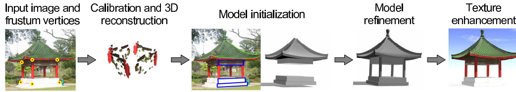
Figure 5.3: The modeling pipeline. We first calibrate the camera according to the user specified frustum vertices and reconstruct a set of 3D points. The architecture components (i.e. walls and roofs) are then interactively decomposed and modeled. Shape details can be added if necessary. Lastly, the final model is textured with the texture enhancement technique described in Section 5.3.2.
