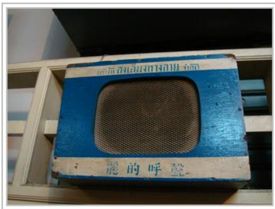
Figure 3.3 Picture of Rediffusion receiving box
