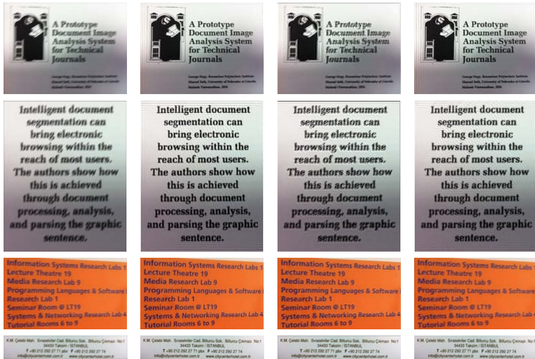
Figure 9.14: Four motion blurred document image examples in the first column and corresponding recovered images by our proposed method in the second column, Shan et al.'s method [9] in the third column and Qi's method [6] in the fourth column, respectively.
