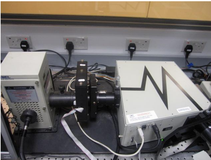
Figure 3-12: IPCE measurement setup using computer monitored monochromator.
