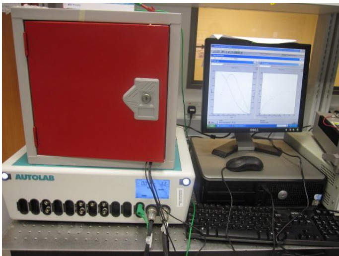
Figure 3-13: Computer monitored Autolab 302N + FRA for impedance measurement.
