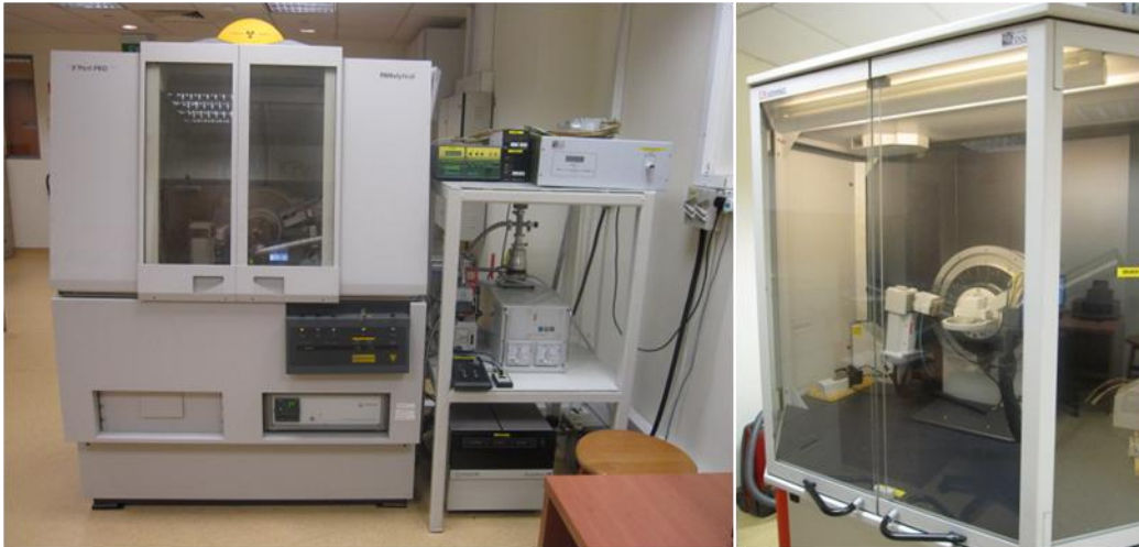
Figure 3-10: X-ray powder diffraction (PANalytical, X'Pert Pro MPD) equipped with a high temperature chamber (ANTON PAAR, HTK 1200) (left); Bruker D8 Advanced Thin Film XRD with incidence angle of 3^\circ (right).
