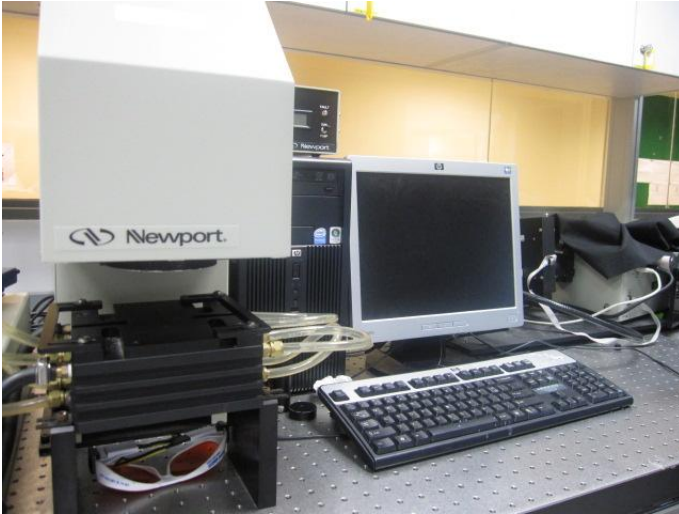
Figure 3-11: JV curve measurement using computer controlled Keithley and solar simulator
