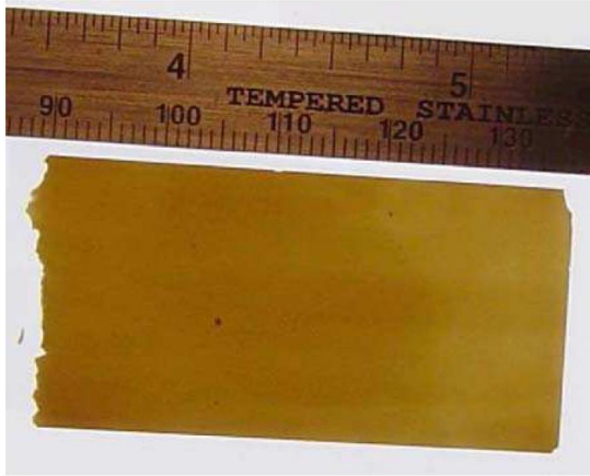
Figure 1-2: A stable, mechanically robust nanotube array membrane after critical point drying. The 200 \mu\text{m} thick membrane, 120 nm pore diameter, is about 2.5 cm \times 4.5 cm [35]
