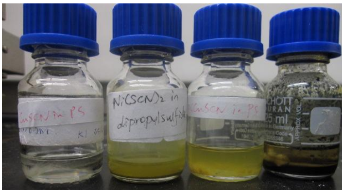
Figure 5-3: From left to right: 0.2 mg CuSCN (transparent), \text{Ni}(\text{SCN})_2 (dark yellow), \text{Cu}(\text{SCN})_2 (light yellow) and THT/CuSCN paste (transparent solution, but paste converts from white to dark after a few days) in propyl sulphide (PS) saturated solution.
