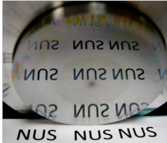
Figure 6.9. Machined surface on hardened stainless steel using a PCD tool with the EVC technology ( DOC = 10 \mu\text{m} , f_r = 2.5 \mu\text{m/rev} , n_r = 15 \text{ rpm} ).
