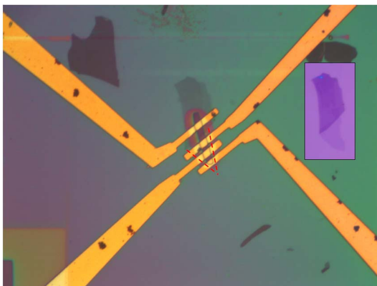
Figure 5.19: Graphene edges covered by a layer of PMMA, with only a portion of the graphene basal plane exposed to a N_2 atmosphere. Red dashed lines indicate the edges of the SLG. Inset: optical image of the graphene flake before device fabrication.
