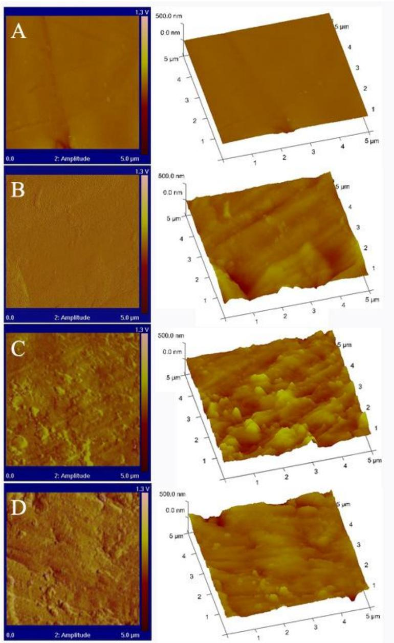
**Figure 6.6** AFM images of (A) pristine CoCr, (B) CoCr-PDOP, (C) CoCr-PDOP BMP2 (10  $\mu$ g/ml) and (D) CoCr-PDOP-BMP Peptide (1000  $\mu$ g/ml) substrates.
