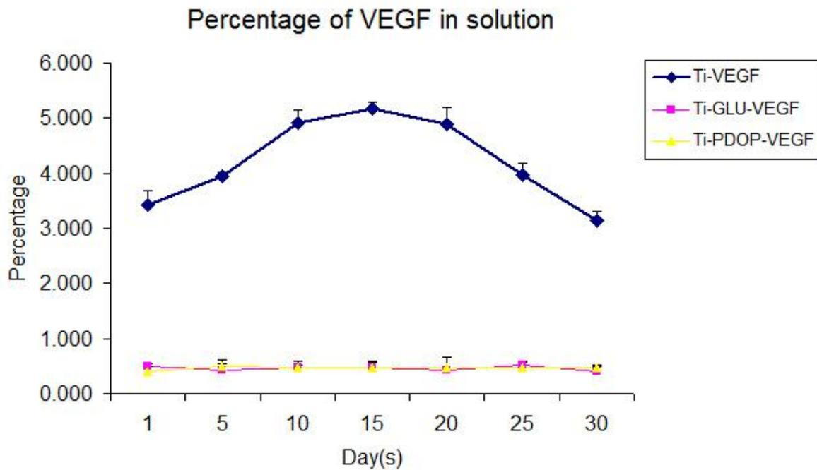
**Figure 3.8** Concentration of VEGF in PBS, expressed as percentage of the initial coating concentration of VEGF on Ti-VEGF, Ti-GLU-VEGF and Ti-PDOP-VEGF substrates ( $n=3$ ). Error bars represent standard deviations
