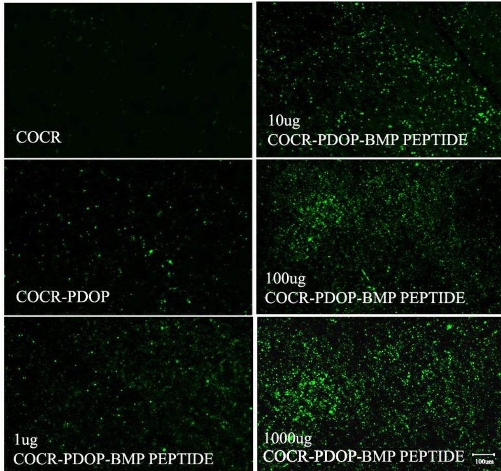
**Figure 6.2** OPA images of pristine CoCr, CoCr-PDOP and CoCr-PDOP-BMP Peptide substrates at various concentrations. The scale bar represents 100  $\mu\text{m}$ .
