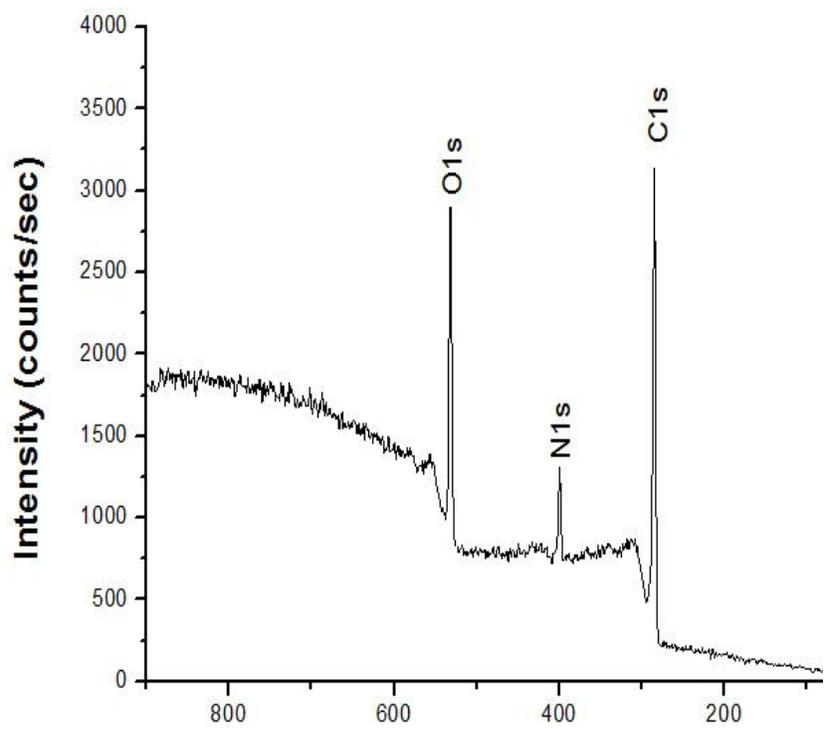
**Figure 3.6** XPS wide-scan spectra of (A) pristine Ti, (B) Ti-VEGF, (C) Ti-GLU-VEGF and (D) Ti-PDOP-VEGF to determine the chemical composition of the surfaces at each stage of modification.
