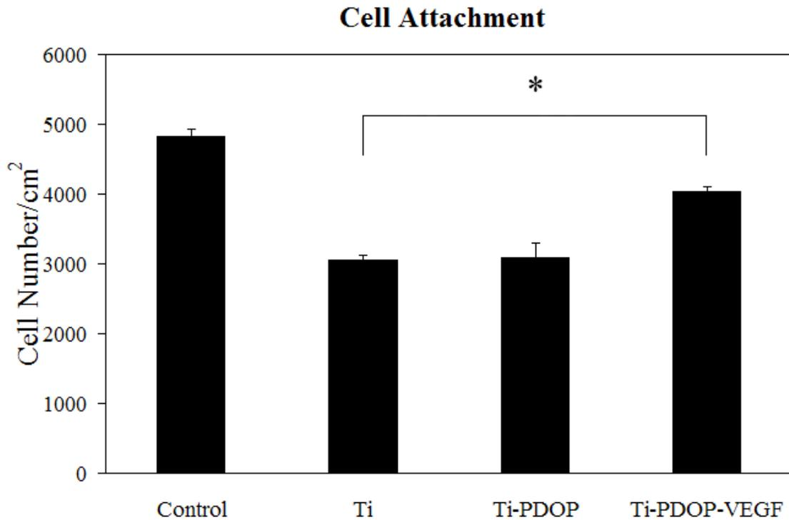
**Figure 4.5** Number of adherent HDMECs per cm<sup>2</sup> on surfaces of control, pristine Ti, Ti-PDOP and Ti-PDOP-VEGF substrates ( $n=5$ ). There is about a 20% increase in HDMEC attachment on the Ti-PDOP-VEGF over the pristine Ti. (\*) denote significant differences ( $P < 0.05$ ) compared with the pristine Ti.
