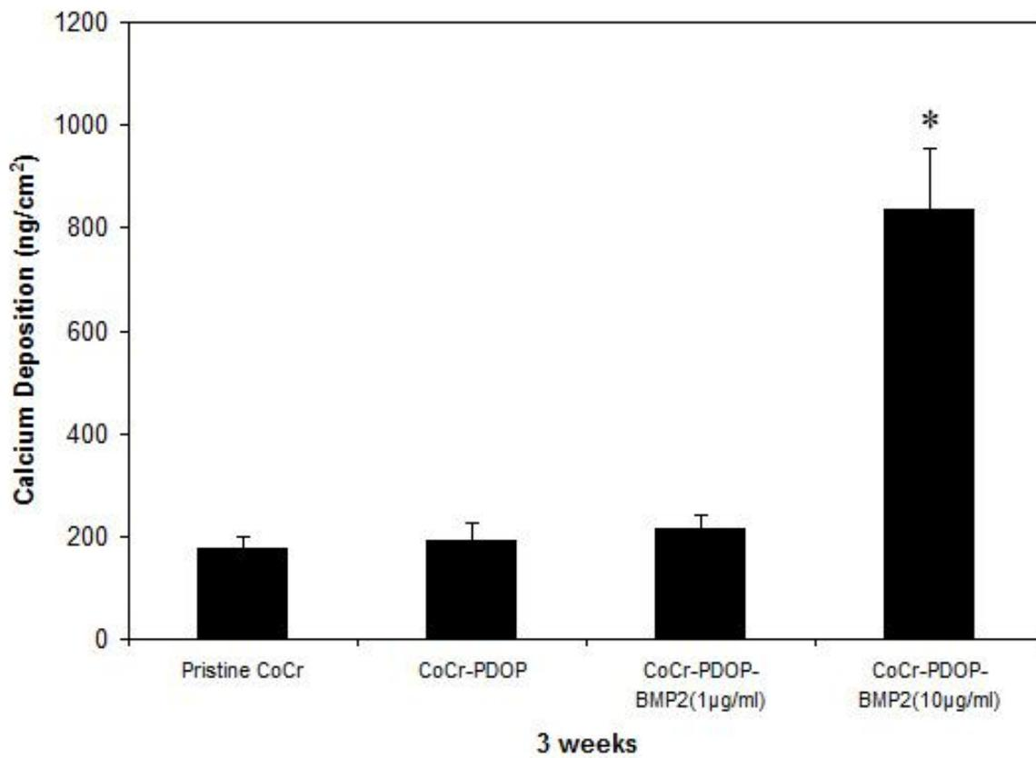
**Figure 5.7** Calcium deposition of MC3T3-E1 seeded on pristine CoCr, CoCr-PDOP, CoCr-PDOP-BMP2 (1 µg/ml) and CoCr-PDOP-BMP2 (10 µg/ml) substrates on week 3 ( $n=3$ ). (\*) denote significant differences ( $P < 0.05$ ) compared with the pristine CoCr.
