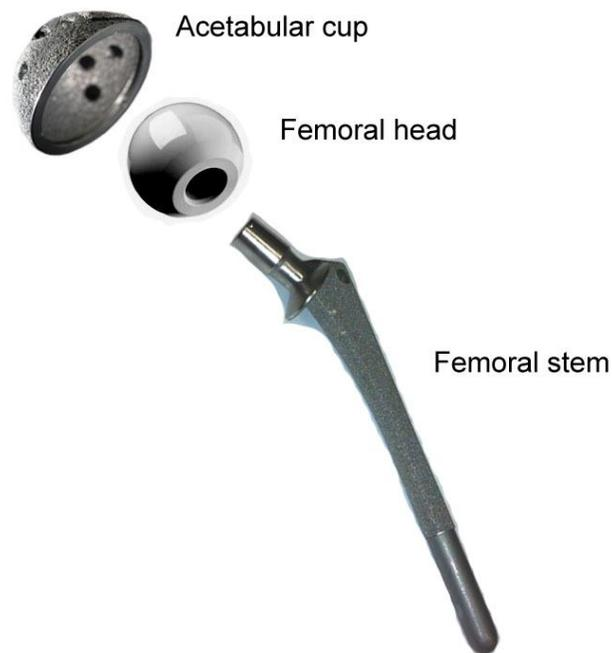
**Figure 2.1** Diagram of a typical hip implant. Acetabular cup and femoral head is usually made of Cobalt Chromium for the bearing strength, while the femoral stem is usually composed of Titanium for the biocompatibility.
