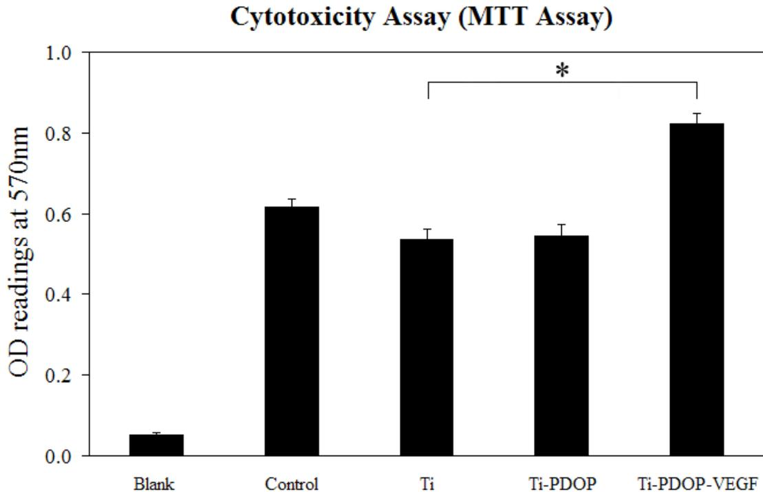
**Figure 4.7** Cell viability measured by MTT assay on the control, pristine Ti, Ti-PDOP and Ti-PDOP-VEGF substrates after 1 week ( $n=5$ ). The assay shows that the substrates do not affect cell viability and there is significantly higher viability of HDMEC observed in the Ti-PDOP-VEGF compared to the pristine Ti. (\*) denote significant differences ( $P < 0.05$ ) compared with the pristine Ti.
