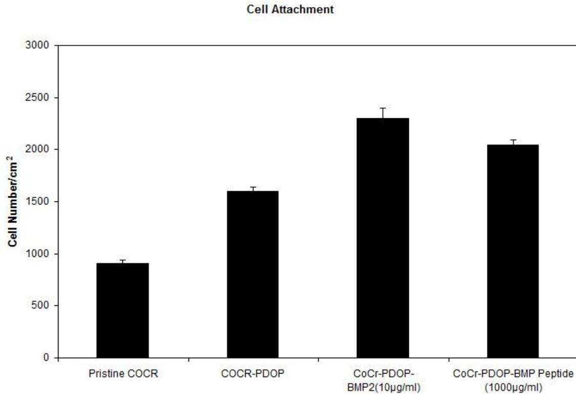
**Figure 6.7** Number of adherent MC3T3-E1 per  $\text{cm}^2$  on surfaces of pristine CoCr, CoCr-PDOP, CoCr-PDOP-BMP2 (10  $\mu\text{g}/\text{ml}$ ) and CoCr-PDOP-BMP Peptide (1000  $\mu\text{g}/\text{ml}$ ) substrates ( $n=3$ ). (\*) denote significant differences ( $P < 0.05$ ) compared with the pristine CoCr.
