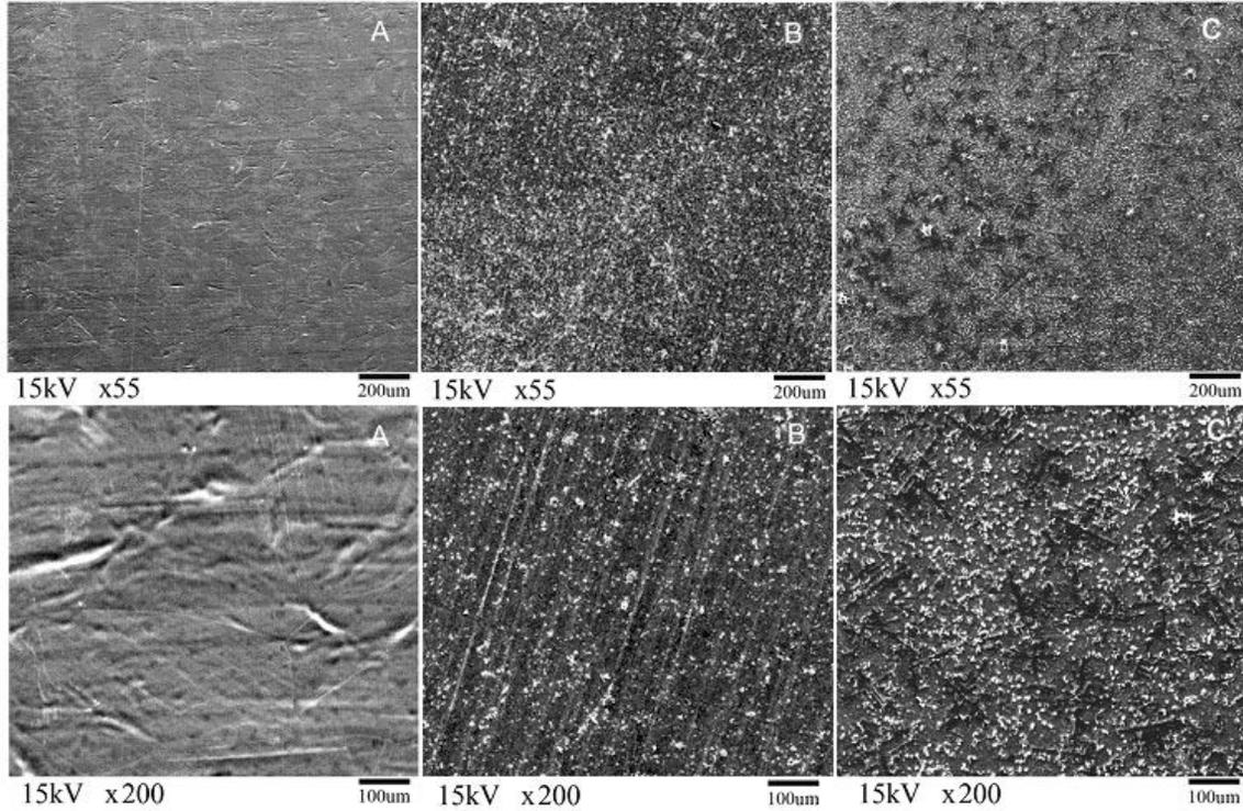
**Figure 4.3** SEM images of (A) pristine Ti, (B) Ti-PDOP and (C) Ti-PDOP-VEGF substrates with different surface properties.
