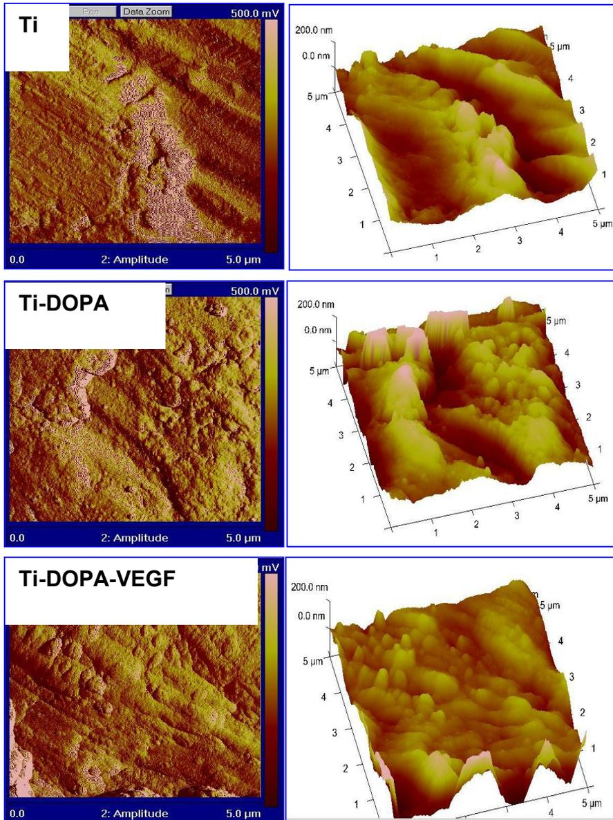
**Figure 4.4** AFM images of (A) pristine Ti, (B) Ti-PDOP, (C) Ti-PDOP-VEGF substrates. There is a general increase in surface roughness of the substrates after each step of modification.
