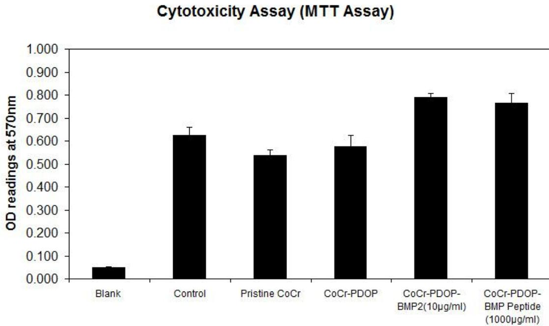
**Figure 6.3** Cell viability measured by MTT assay on the pristine CoCr, CoCr-PDOP, CoCr-PDOP-BMP2 (10  $\mu\text{g/ml}$ ) and CoCr-PDOP-BMP Peptide (1000  $\mu\text{g/ml}$ ) substrates after 1 week ( $n=3$ ).
