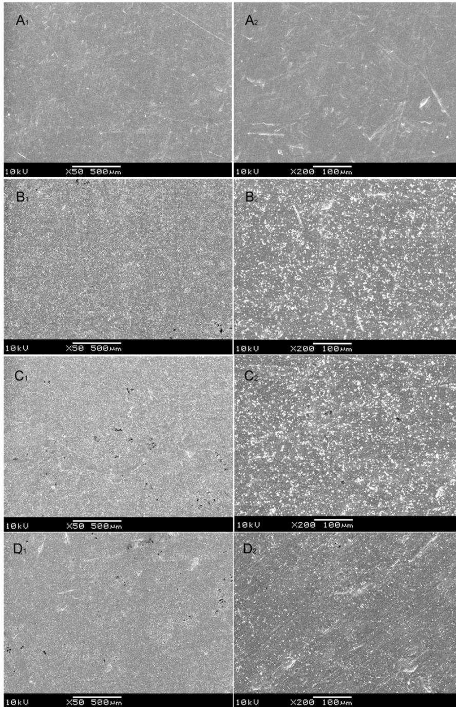
**Figure 6.5** SEM images of (A) pristine CoCr, (B) CoCr-PDOP, (C) CoCr-PDOP BMP2 (10 μg/ml) and (D) CoCr-PDOP-BMP Peptide (1000 μg/ml) substrates.
