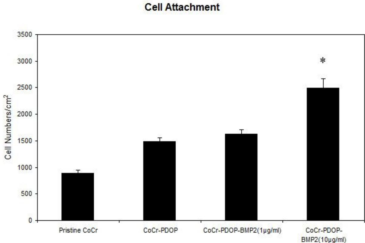
**Figure 5.4** Number of adherent MC3T3-E1 per  $\text{cm}^2$  on surfaces of pristine CoCr, CoCr-PDOP, CoCr-PDOP- BMP2 (1  $\mu\text{g/ml}$ ) and CoCr-PDOP-BMP2 (10  $\mu\text{g/ml}$ ) substrates ( $n=3$ ). (\*) denote significant differences ( $P < 0.05$ ) compared with the pristine CoCr.
