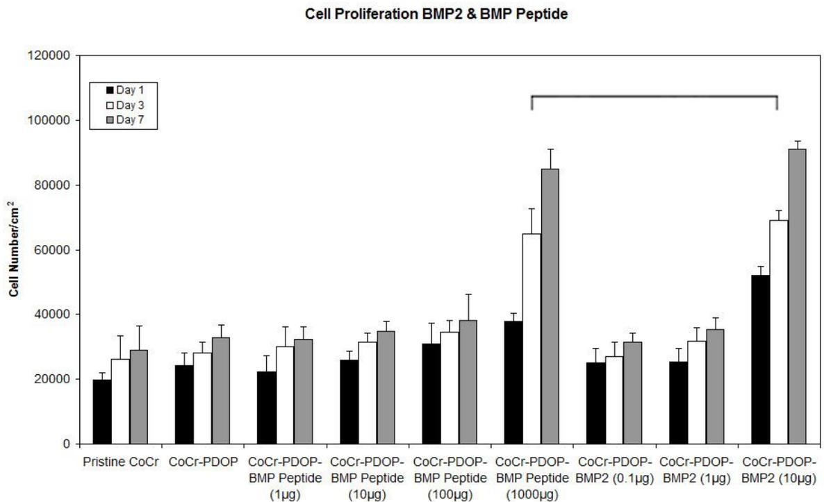
**Figure 6.1** Comparison of MC3T3-E1 proliferation over 7 days on surfaces of control, pristine CoCr, CoCr-PDOP-BMP Peptide and CoCr-PDOP-BMP2 substrates at various concentrations on days 1, 3 and 7 ( $n=3$ ).
