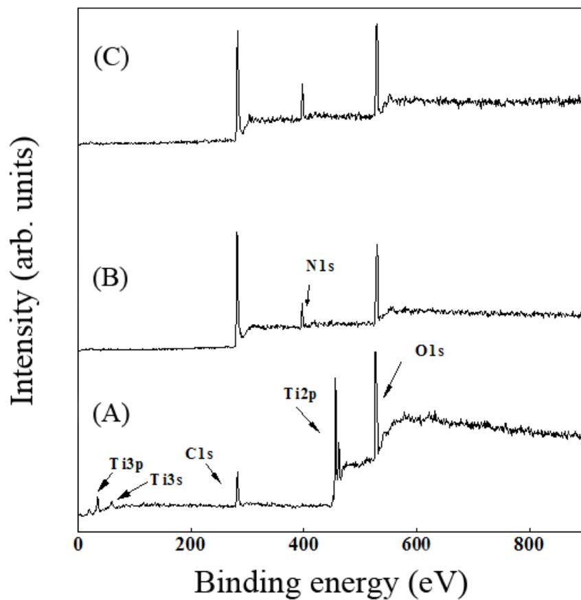
**Figure 4.2** XPS wide-scan spectra of (A) pristine Ti, (B) Ti-PDOP and (C) Ti-PDOP-VEGF to determine the chemical composition of the surfaces at each stage of modification.
