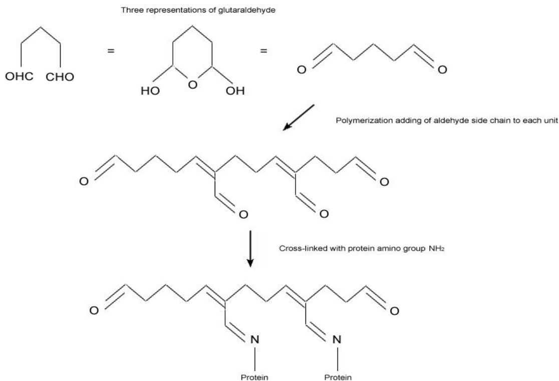
**Figure 3.3** Schematic diagram showing glutaraldehyde cross-linking with proteins.
