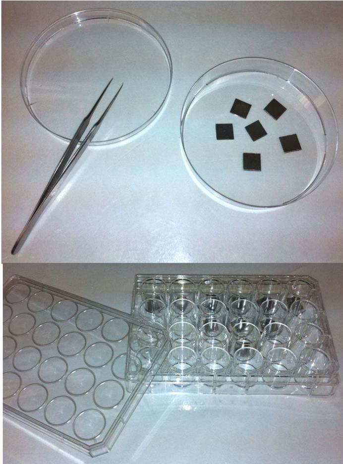
**Figure 3.2** Substrates preparation to 1 cm by 1 cm and placing them in 24 well plates for subsequent experiments.
