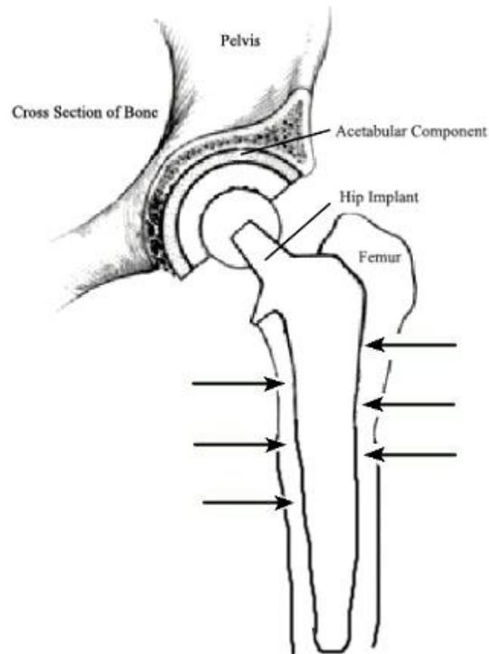
**Figure 4.1** Schematic figure of a hip resurfacing implant: hemispherical cobalt chrome alloy component capping onto the femoral head of the hip joint, with Titanium guide stem inserted in femoral neck region. The femoral neck is the region at risk of compromised vascularity. Arrows indicate area of compromised vascularity.
