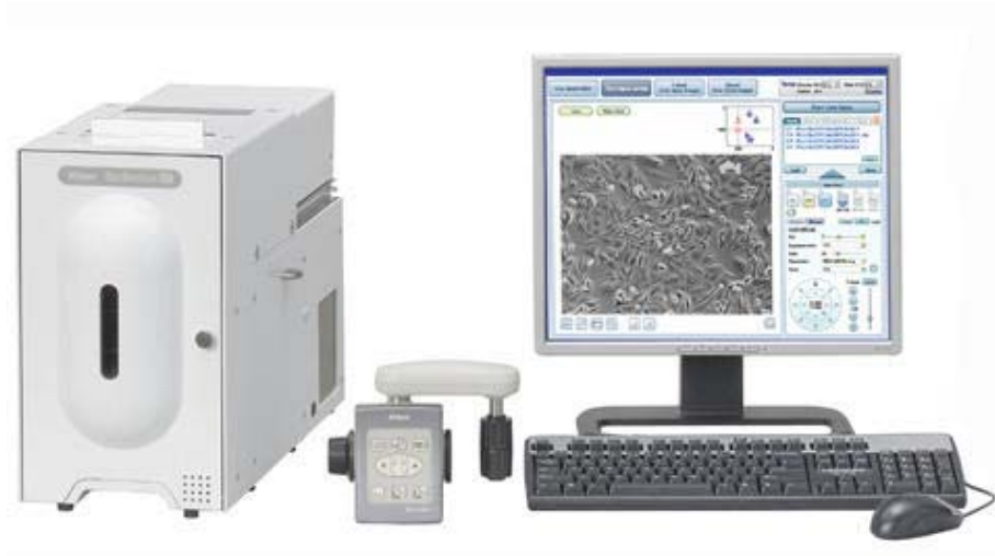
Figure 3.3 The Biostation IM (Nikon). The white box on the left resembling a Central Processing Unit (CPU) actually hosts the motorized microscope, incubation chamber with immobile stage and the humidifier unit. The unit in the center is the controls for the movement of the microscope objectives (10X, 20X and 40X) equivalent to the x-y-z axis movement of a usual microscope stage. The monitor shows the proprietary software used to manipulate the Biostation. The CPU is hidden from the view. ( www.nikoninstruments.com )
