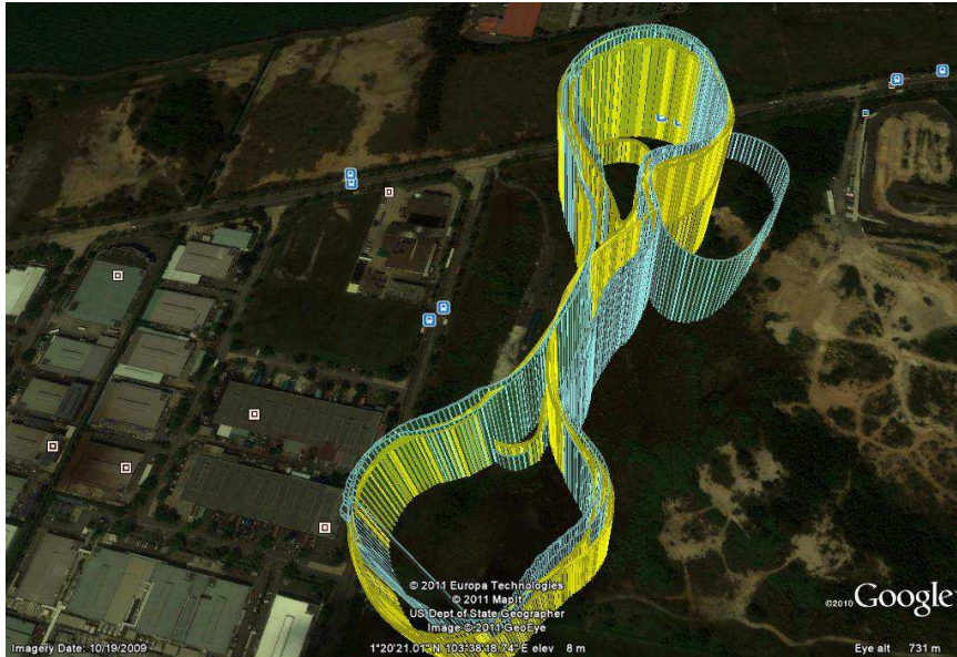
Figure 10.14: Telemetry plot of flight paths with PID (blue) and DCS (yellow) based controllers for third run in straight line tracking tests
