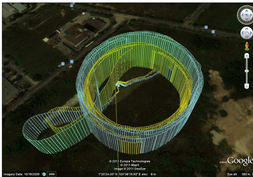
(b) Telemetry plot of flight paths with PID (blue) and DCS (yellow) based controllers
