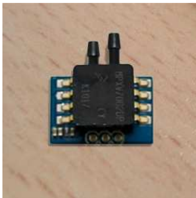
(a) MPXV7002 airspeed sensor
