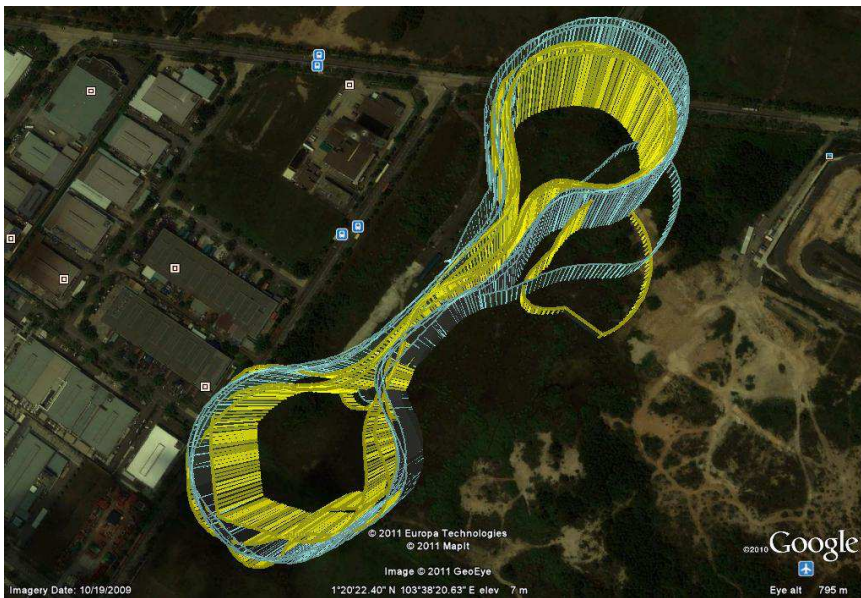
Figure 10.13: Telemetry plot of flight paths with PID (blue) and DCS (yellow) based controllers for second run in straight line tracking tests
