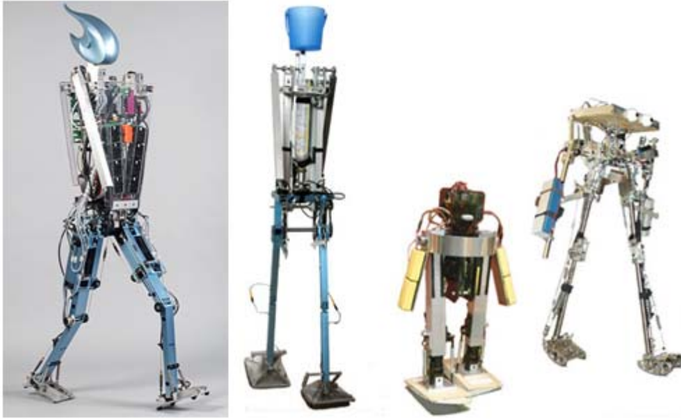
Figure 6: Passive bipedal robots. From left to right: Flame and Denise by TU Delft, Toddler by Massachusetts Institute of Technology, and The Cornell Biped by Cornell University.
