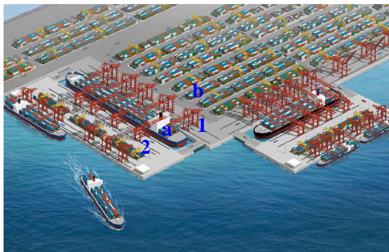
Figure 5.1: Hybrid quay wall proposed for the west terminal of Busan New Port
