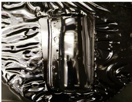
Fig. 4.8: Peeling-off the membrane: The picture shows how membrane is peeled-off from the master-mold using IPA. The film is automatically released from the mold if it is kept at 70°C for about 30min.
