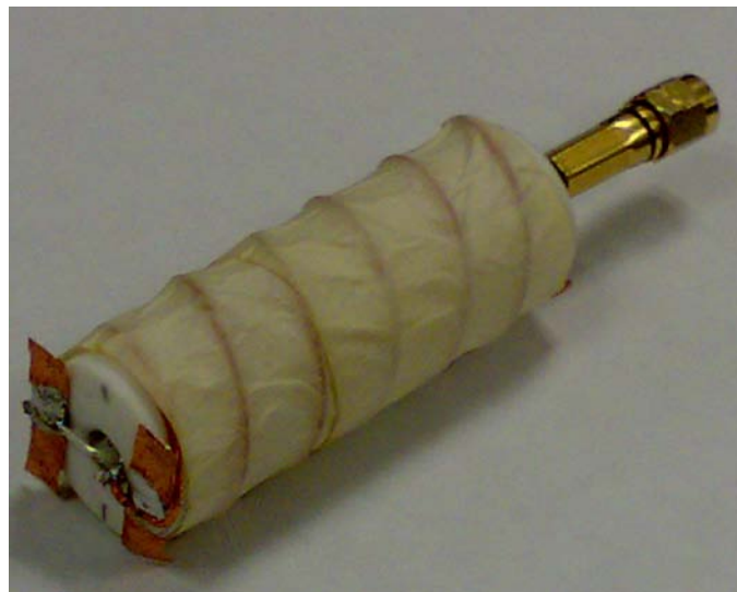
Figure 3.2 The image of the dielectric-loaded bifilar backfire helical antenna.
