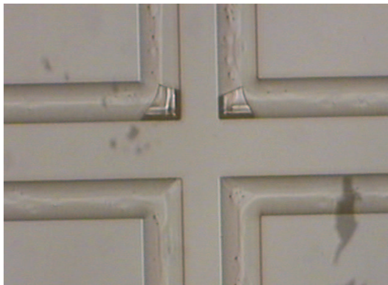
Figure 6.10. PR peel off due to long time wet etching
