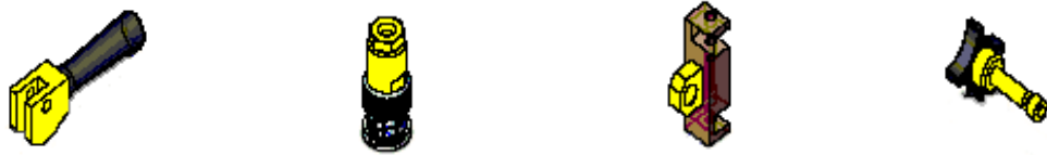
Figure 6-11. Mechanically meaningful sub-parts (colored in yellow) extracted by the proposed semantic-based decomposition
