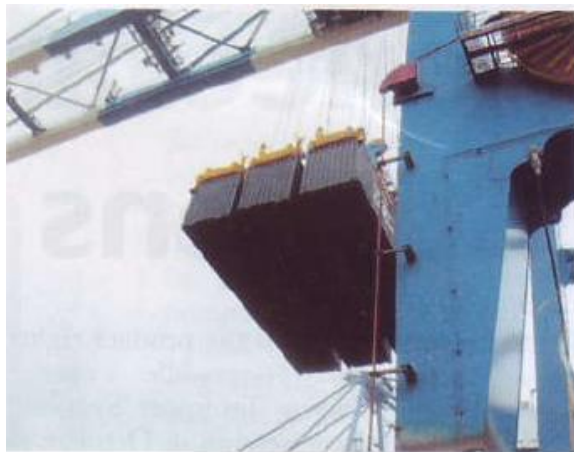
Figure 1.5: Triple lift quay crane, able to carry three 40-footers together
