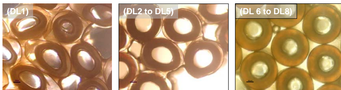
Figure 4.3. Effects of non-solvent additives on the delamination of the dual-layer hollow fiber membranes (Scale bar 50 \mu m). (a) DL1 (Outer layer: PAI/NMP:27/73; inner layer: CA/NMP:16/84); (b) DL2 to DL5 (Outer layer: PAI/NMP:27/73; inner layer: CA/NMP/additive/Mg(ClO 4 ) 2 =16/67.5/15/1.5); (c) DL6 to DL8 (Outer layer: PAI/NMP/additive:27/63/10; inner layer: CA/NMP/additive/Mg(ClO 4 ) 2 =16/67.5/15/1.5).
